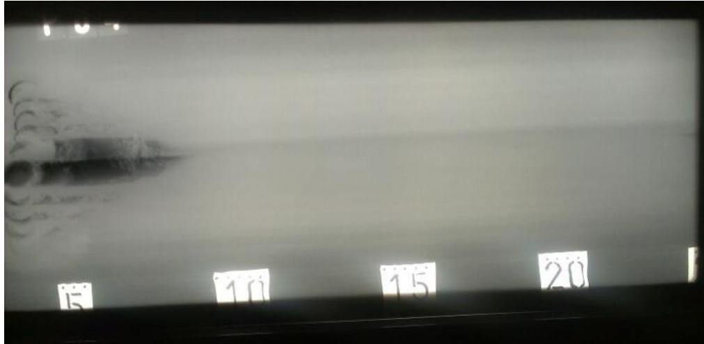
Figure 4-15. Radiograph of the plate having overlapped FSP lines (290 rpm, 100 mm/min)
