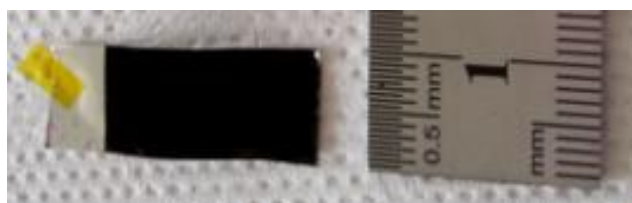
Figure 4.2 Photograph of a CNT/aluminum foil electrode sample.
