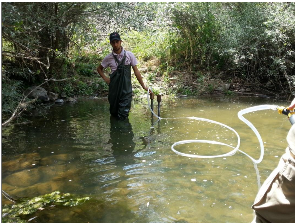
Figure 20: Purging of deep piezometer in S4-P site for measurement of water quality field parameters.
