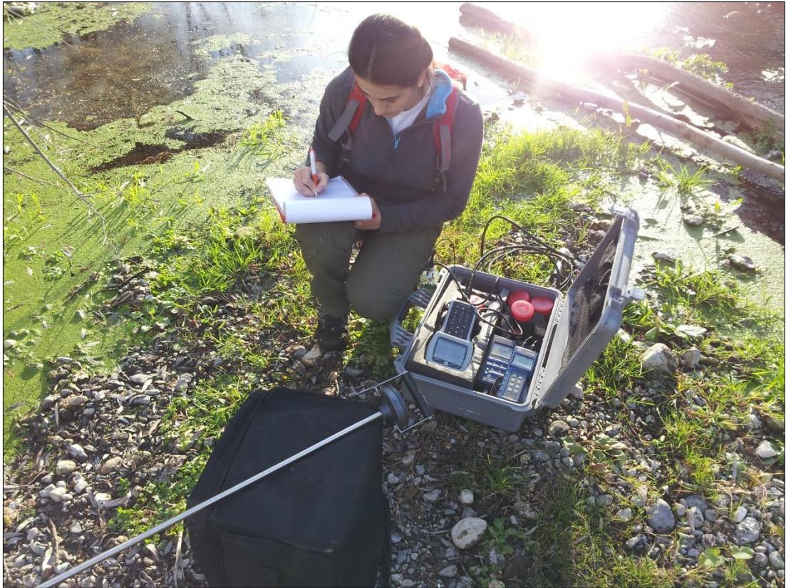
Figure 19: Measurement of water quality field parameters for stream water in the field.
