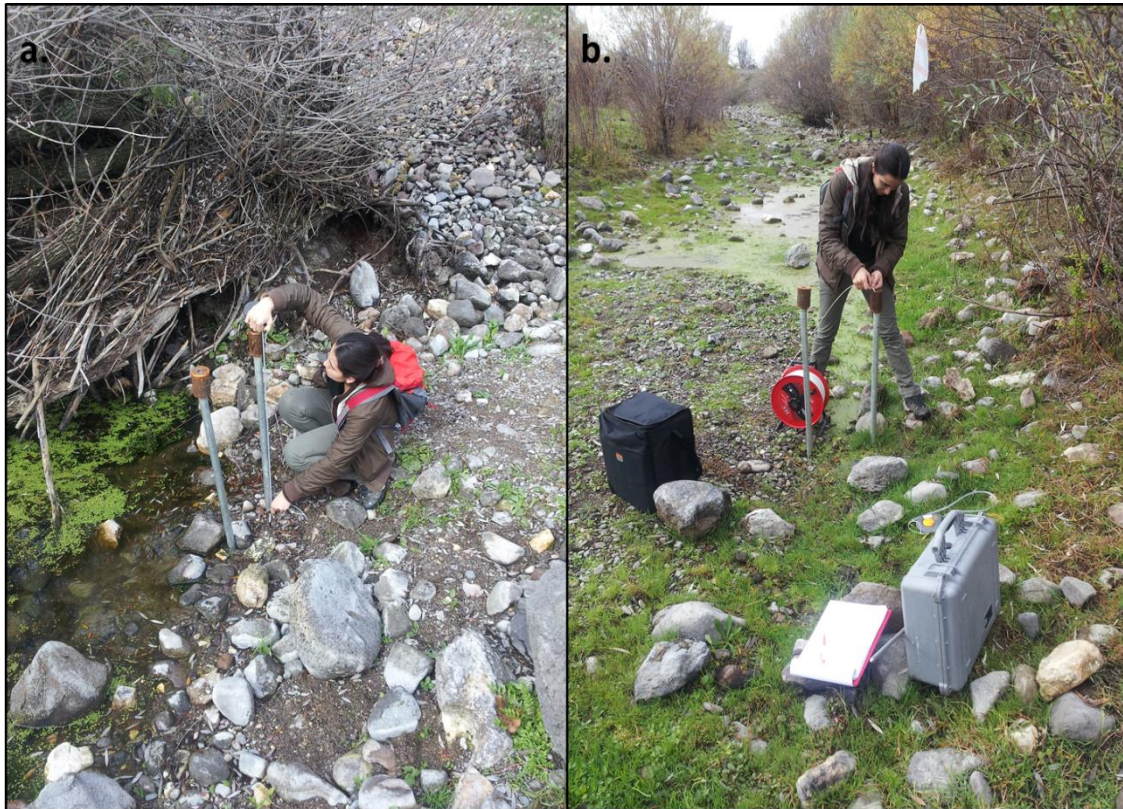
Figure 15: a) Nested piezometers and measurement of height of the piezometer above ground b) Measurement of water levels inside the nested piezometers by Solinst TLC Meter.
