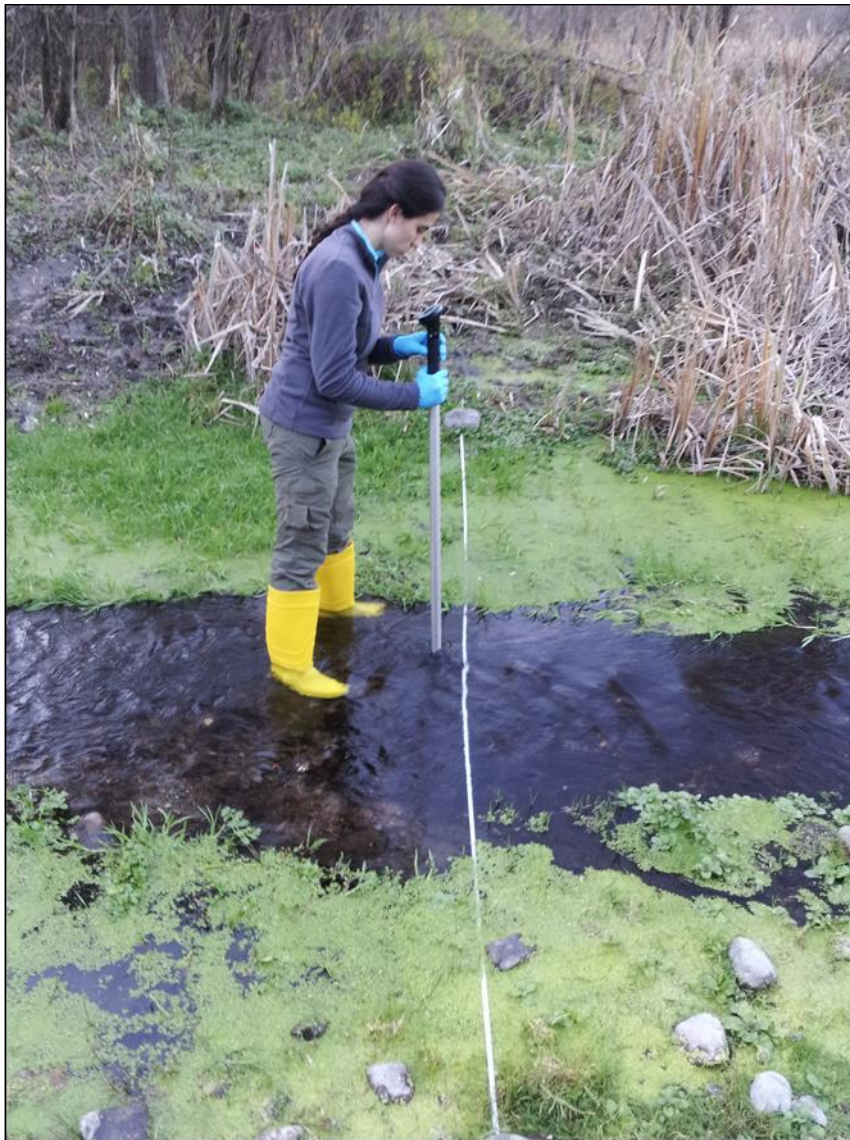
Figure 17: Measurement of discharge by FP111 Globe Water Flow Probe in monitoring location S17-D.
