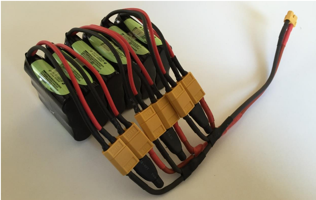
Figure 6.7: Final Battery Stack of ALM
