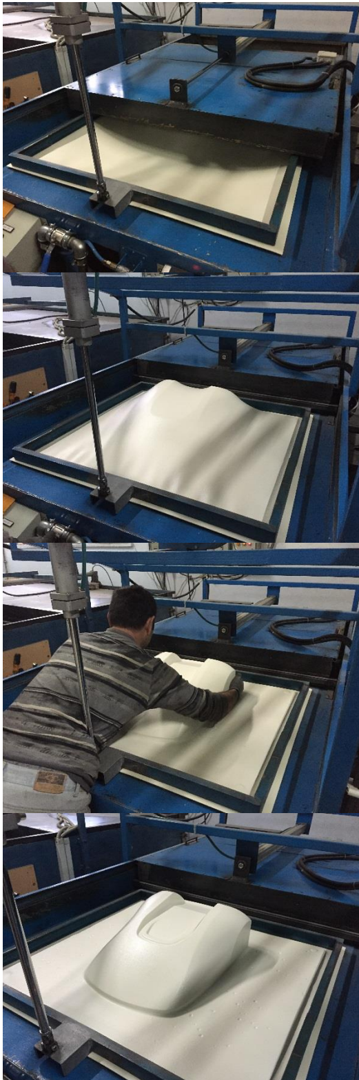
Figure 6.4: Production Stages of Outer Cover
