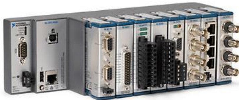
Figure 47: National Instruments Compact RIO 9066 Chassis [23]
