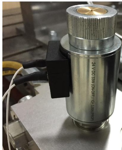
Figure B. 2: Proportional Pressure Relief Valve
