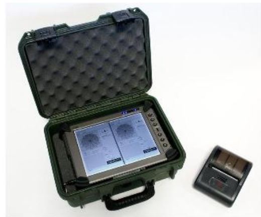
Figure 1.2 Acoustic Miss Distance Indicator used by Meggit Defence Systems [21]
