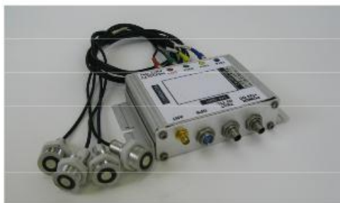
Figure 1.2 Acoustic Miss Distance Indicator used by Meggit Defence Systems [21]
