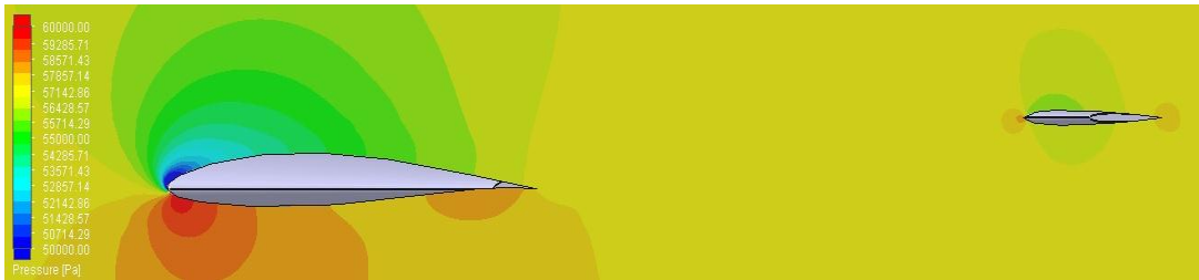
Figure 4.46 Pressure Contour Cut plots 0.231m from centerline of T-tail, Cruciform tail and Conventional Tail at \alpha=14^0
