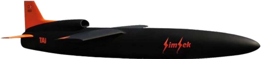
Figure 1.4 Şimşek High Speed Decoy UAV Designed by TAI [18]
