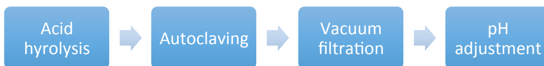
Figure 3.1 Schematic of one-step acid pretreatment
