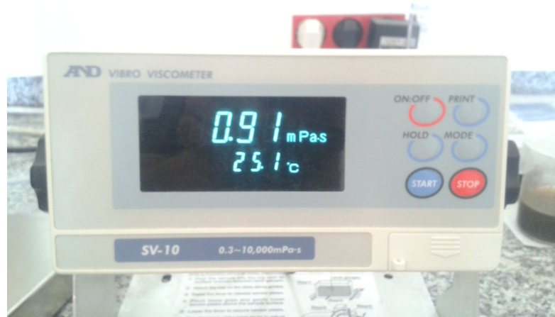
Figure 2.12: A&D SV-10 vibro viscometer
