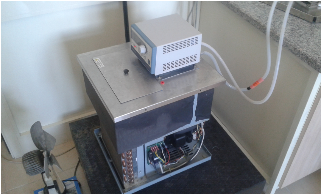
Figure 2.13: Constant temperature water provider for viscometer
