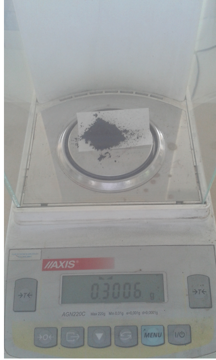
Figure 2.17: Spilling of CNTs during weighing
