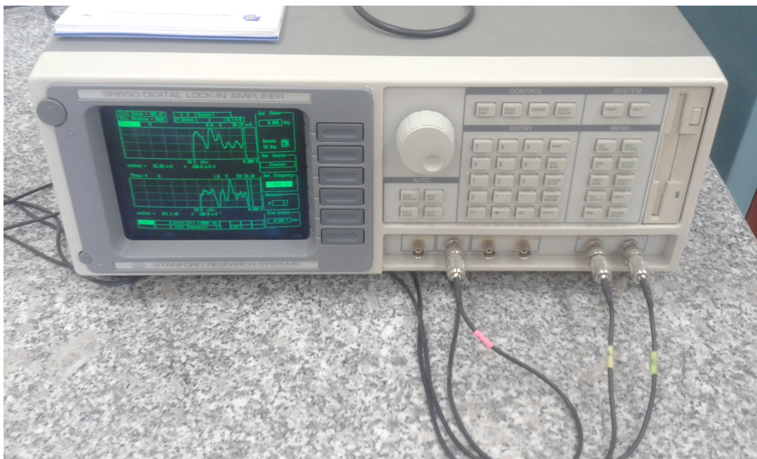
Figure 2.8: Stanford SR850 digital lock-in amplifier
