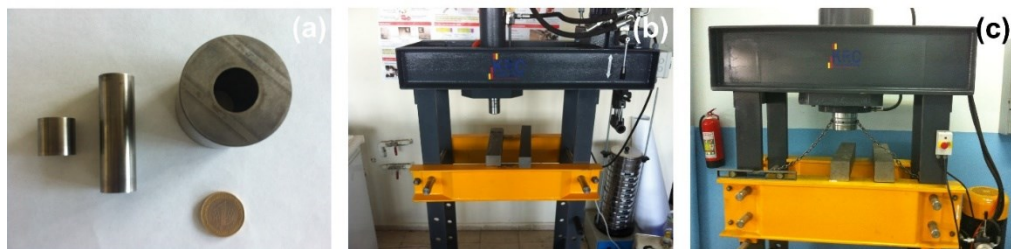
Figure 3.2: (a) A 15mm diameter die used for pressing experiments. (b)-(c) The hydraulic presses used for the experiments having 30 and 300 tons of maximum loads, respectively.
