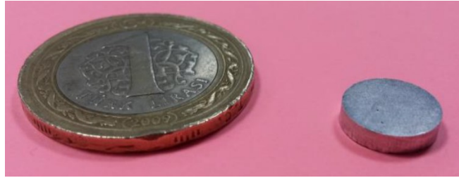
Figure 3.29: An ex-situ composite sample, produced with warm pressing.
