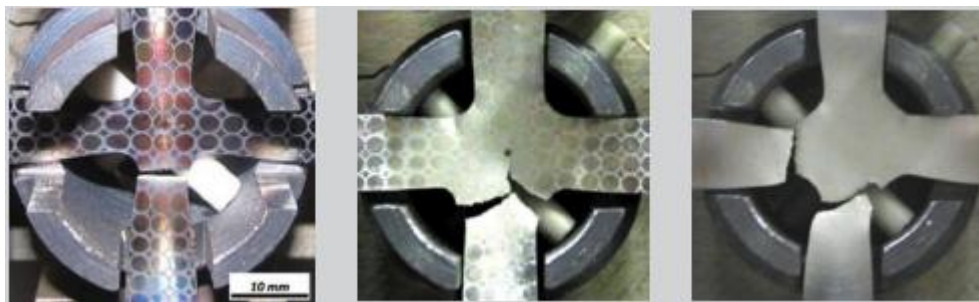
Figure 2.9. Fractured cruciform specimens [44].
