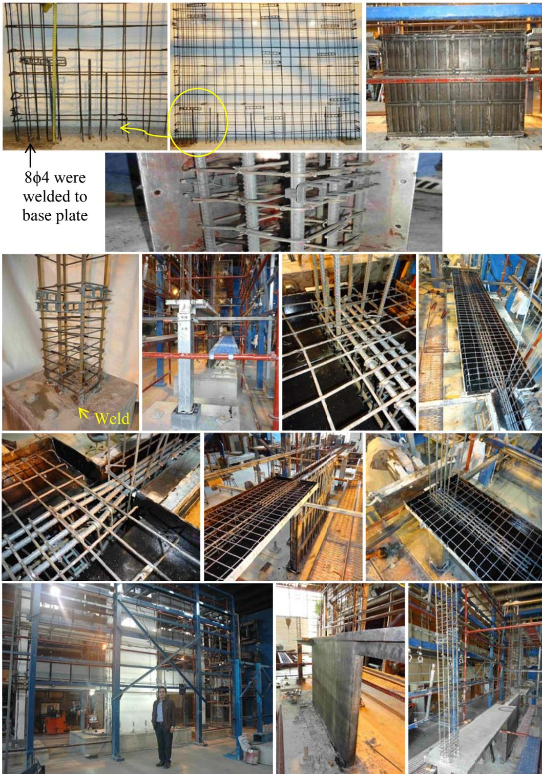
Figure 3.15 Construction stages of RC-SW2
