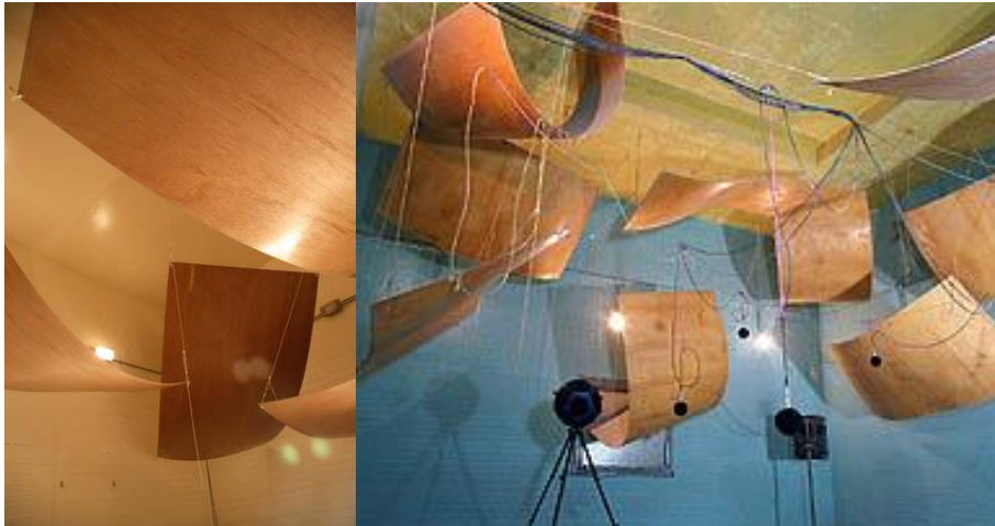
Figure 2.8: Reflective plates and a reverberation chamber. Image courtesy of University of Salford.
