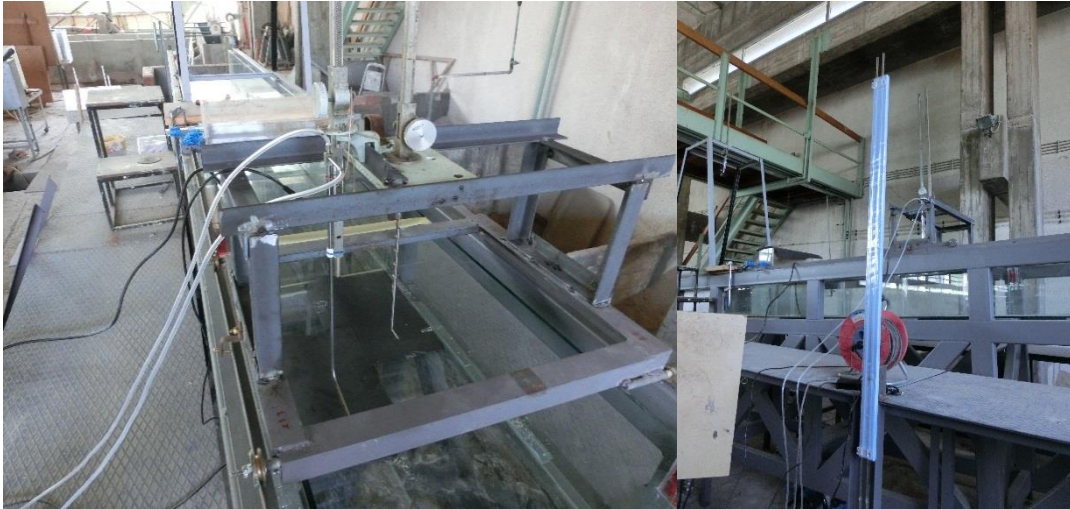
Figure 2-13 : Monometer (left), Pitot tube and the Hot-film probe in operation
