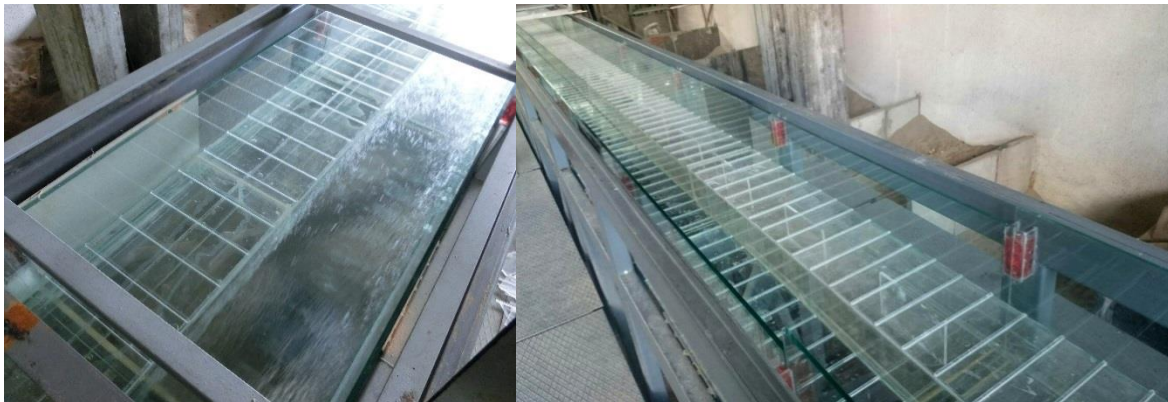
Figure 2-9 : Floodplain rough (left picture) and all bed rough (right picture) compound channel
