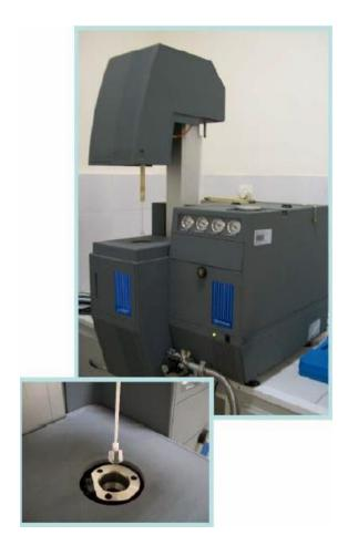
Figure 3.3 DSC used in isochronal thermal analysis.
