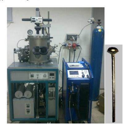
Figure 3.2 Suction casting unit and rod shaped specimen.
