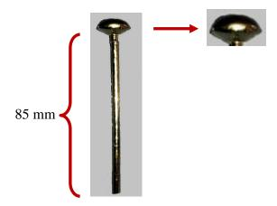
**Figure 4.4** Investigated head part of the bulk glassy (Fe<sub>36</sub>Co<sub>36</sub>B<sub>19.2</sub>Si<sub>4.8</sub>Nb<sub>4</sub>)<sub>99.25</sub>Cu<sub>0.75</sub> alloy for homogenity.
