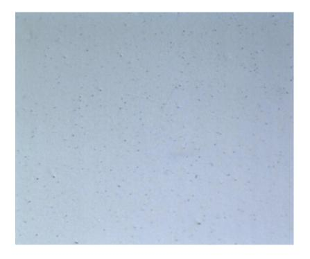
$\label{eq:Figure C.1} \textbf{Figure C.1} \ \text{Optic microscope image of the } \\ (\text{Fe}_{36}\text{Co}_{36}\text{B}_{19.2}\text{Si}_{4.8}\text{Nb}_4)_{99.25}\text{Cu}_{0.75} \ \text{alloy} \\ \\ \text{annealed isothermally at 535 °C.}$
