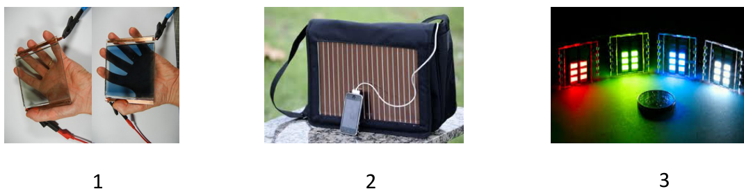
Figure 1.11: 1. Electrochromic device, 2. organic photovoltaic, 3. organic light emitting diode.
