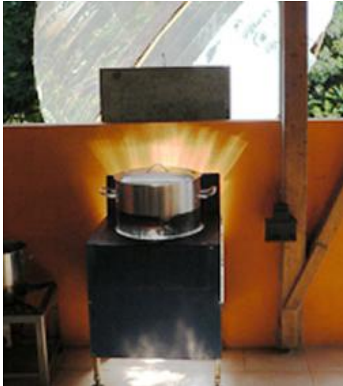
Figure 4.7. Baking oven heated by the Scheffler Mirror in Tamera ( http://www.tamera.org/project-groups/autonomy-technology/scheffler-reflector/ )
