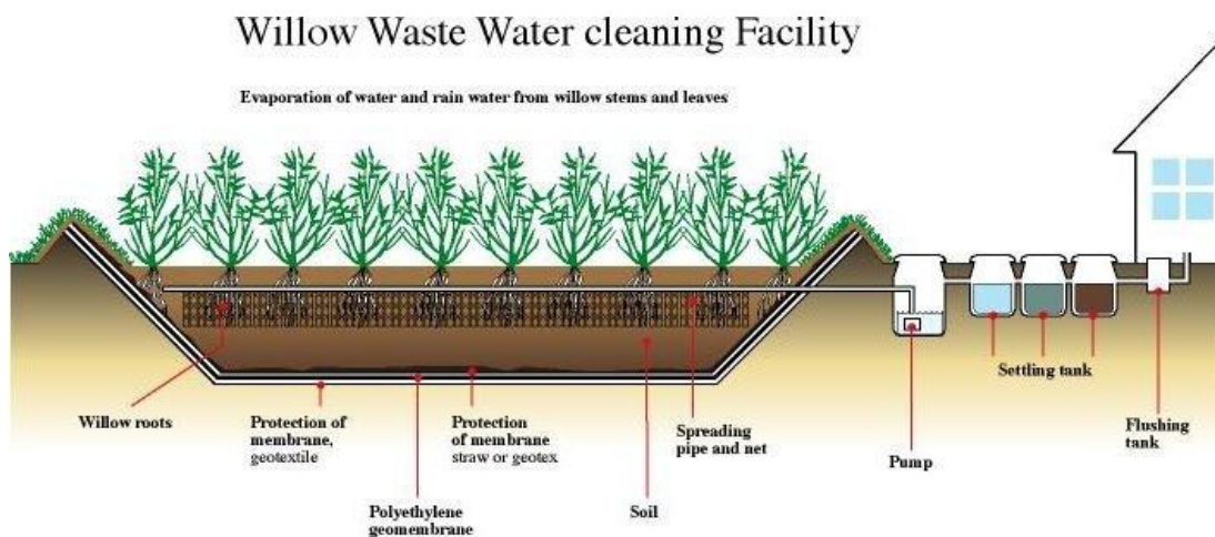
Figure 4.10. Depiction of Willow Waste Water Treatment System http://www.pilerensning.dk/english/index.php?option=com_content&view=article&id=53&Itemid=56&lang=en
