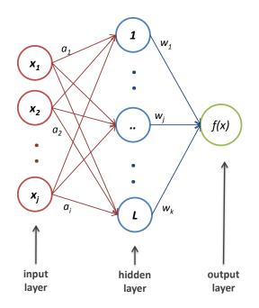
Figure 4.3: Feedforward neural network with a single hidden layer.
