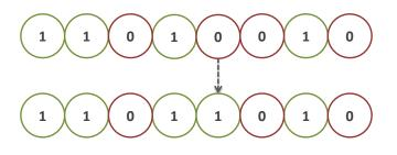
Figure 3.4: Bit flip mutation operation.
