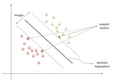
Figure 4.1: Separating two classes by constructing a hyperplane with Support Vector Machines.
