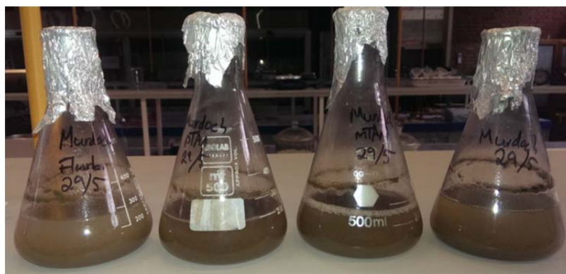
Figure 4. 1. Four enrichments immediately following amendment with, respectively, FLB, pTAA, mTAA, and no amendment.
