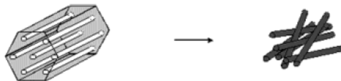
Figure 4.8: Absence of interconnecting micropores in MCM-41 leading to disordered mesoporous-microporous structure after nanocasting process (adapted from Ryoo et al. , 2001)
