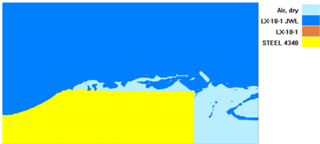
Figure 4-13 Simulation Model of Dent Test
