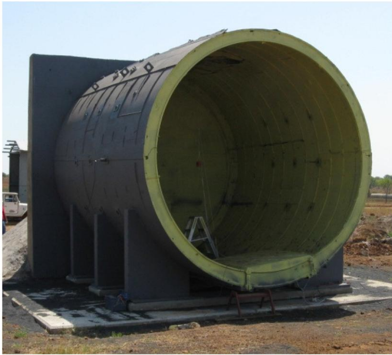
Figure 2-4 Semi-Confined Space to See the Effects of Confinement [6]
