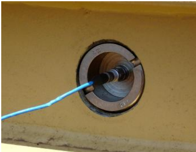
Figure 2-8 Reflected Pressure Sensor to Measure the Pressure [7]
