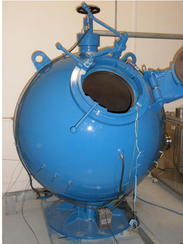
Figure 3-1 Laboratory Detonation Chamber Body Located at ROKETSAN A.Ş.
