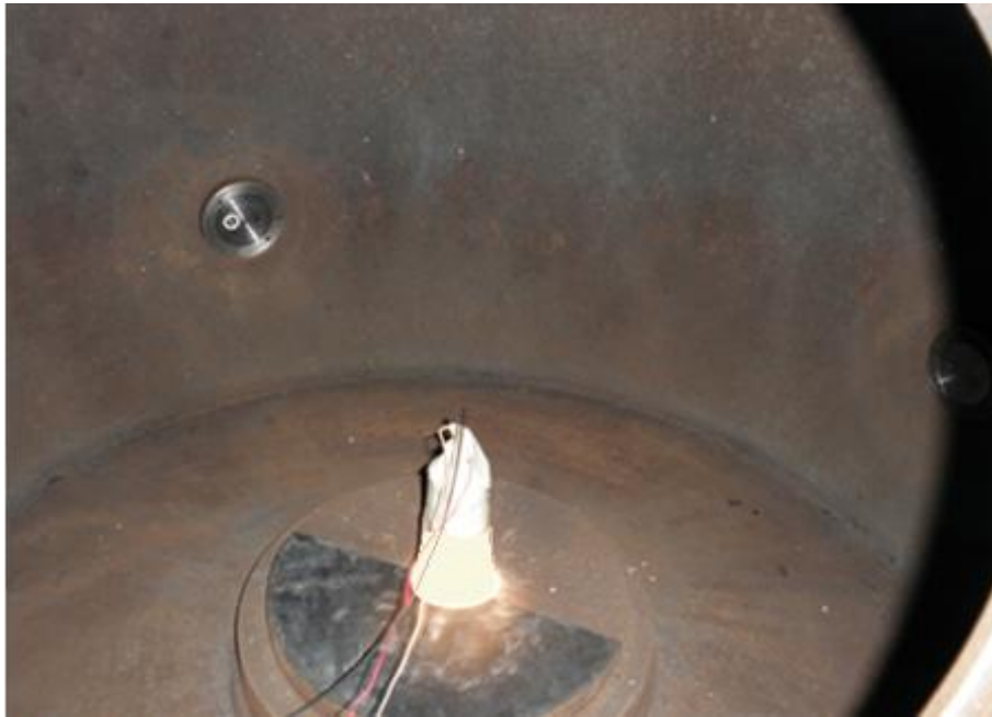
Figure 3-8 Positioned Charge Assembly with the Base Plate
