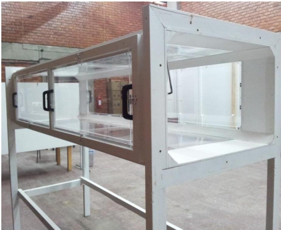
Figure 3.2 Optically transparent test section
