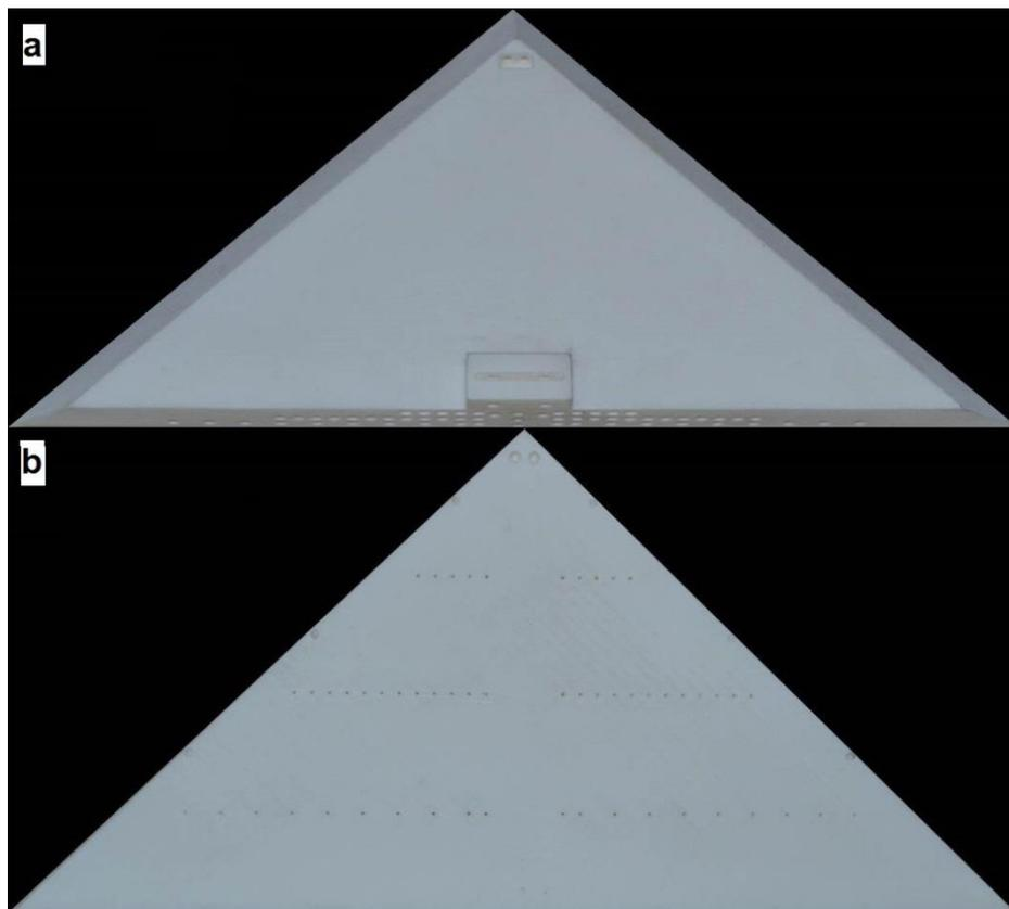
Figure 3.8 Photographs of the fabricated delta wing from different views; a) Top-back view, b) Bottom view, which also shows the pressure taps that were used in pressure measurements
