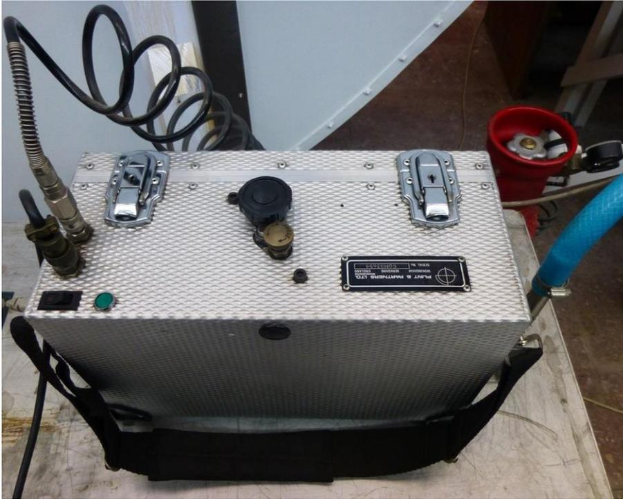
Figure 3.9 The smoke generator used in experiments (Plint&Partners Como3694)
