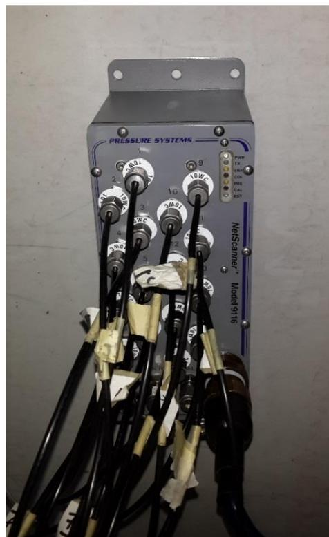
Figure 3.12 The 16-channel pressure scanner system used in the experiments (Netscanner 9116)
