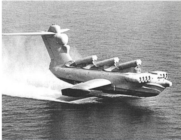
Figure 1-5: An example of ground effect vehicles “Ekranoplan” [13]
