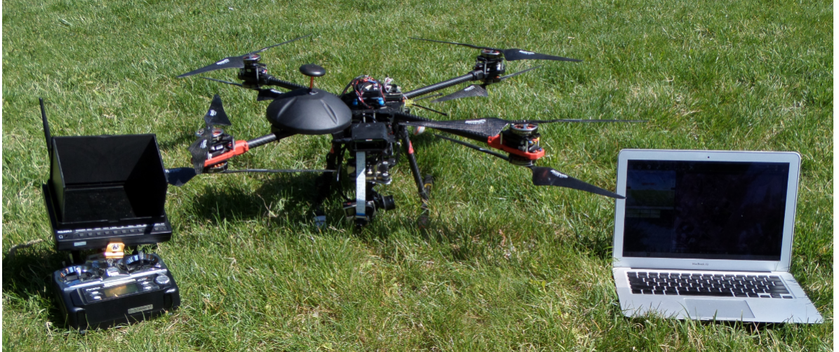
Figure 6.37: Quadcopter, controller and mission planner program
