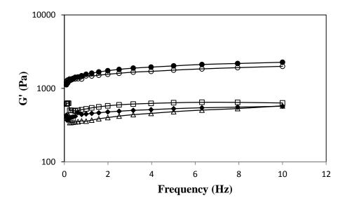
**Figure 3. 9** Storage modulus (G') of batter samples with 10% carob bean flour: xanthan gum ( $\bullet$ ), guar gum ( $\circ$ ), soy protein ( $\Box$ ); whey protein ( $\Delta$ ), control ( $\bullet$ )
