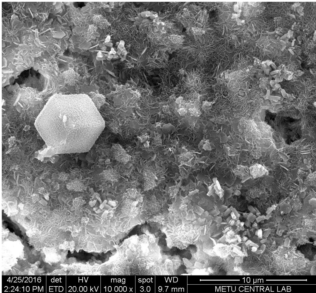
Figure 32: SEM image of A3.1150.2+6% paste at 2 days of hydration.
