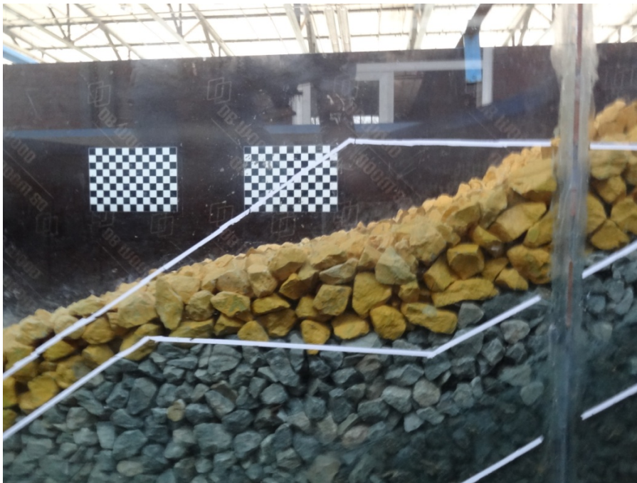
Figure 4.21: Set-1 of Model 2 cross-section after the test
