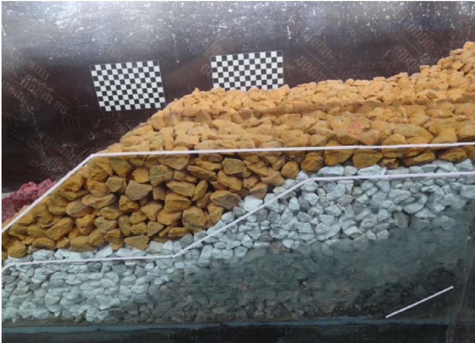
Figure 4.22: Set-1 of Model 3 cross-section before the test
