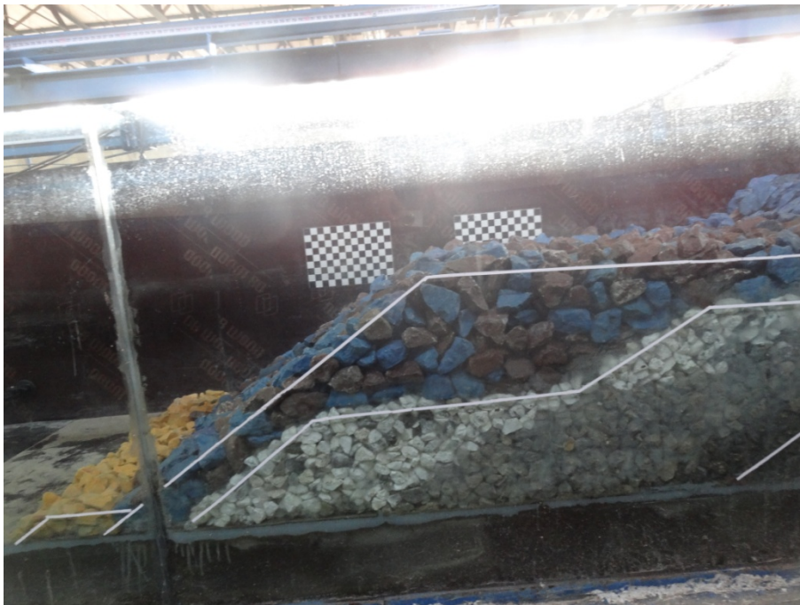
Figure 4.26: Set-2 of Model 5 cross-section before the test
