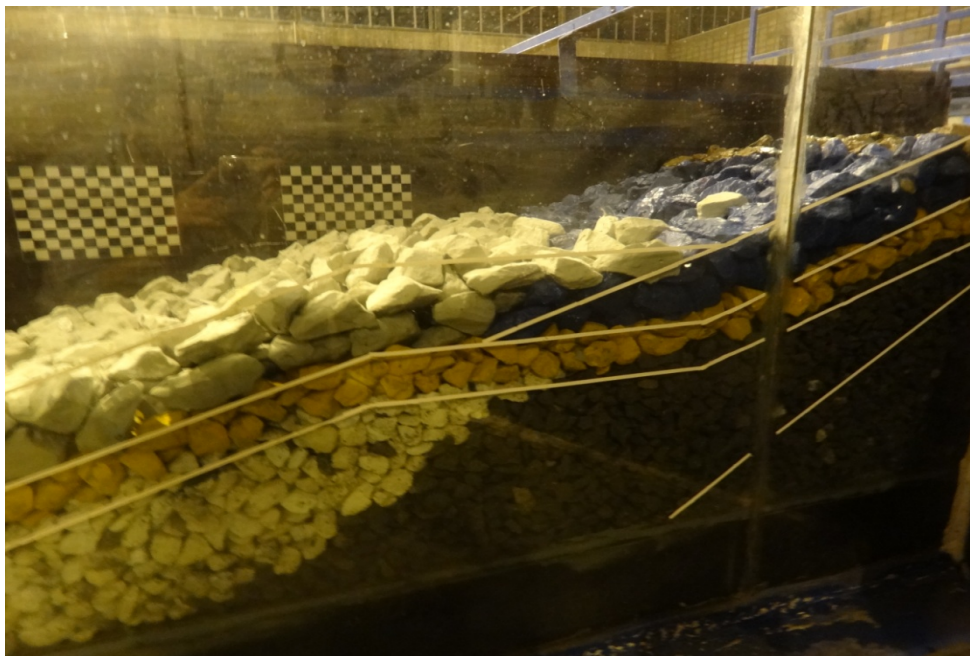
Figure 4.19: Set-1 of Model 1 cross-section after the test
