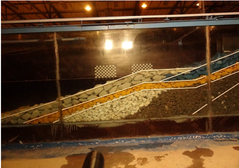
Figure 4.18: Set-1 of Model 1 cross-section before the test
