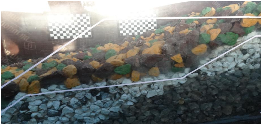
Figure 4.30 View of Section 4 after set 3 (10000 waves)
