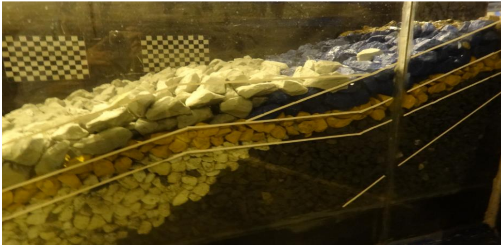
Figure 4.2 View of Section 1 after Set 1 (1000 waves)
