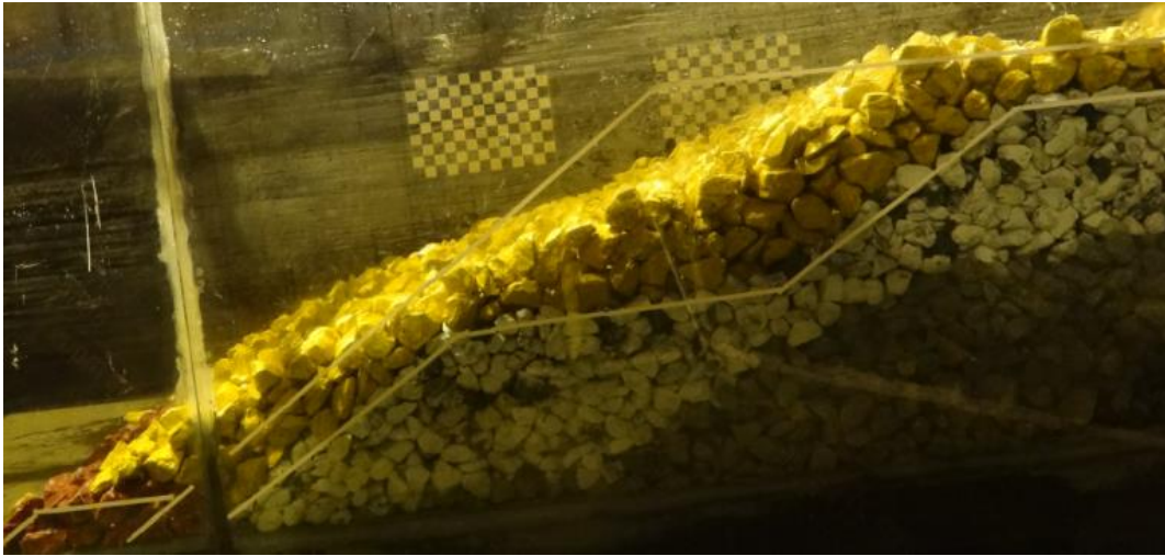
Figure 4.19 View of Section 3 after set 1 (1000 waves)
