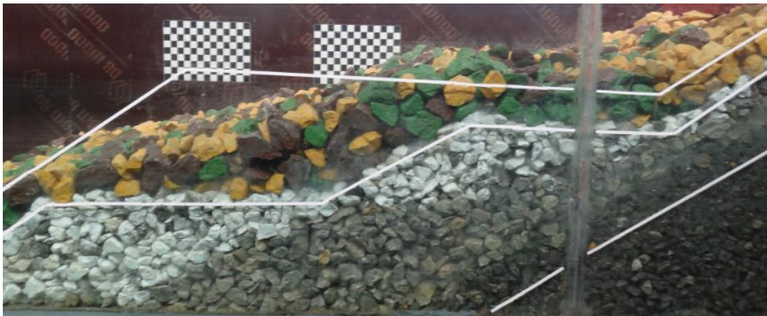
Figure 4.28 View of Section 4 after set 3 (4000 waves)
