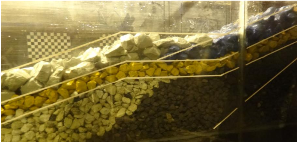
Figure 4.5 View of Section 1 after Set 3 (5000 waves)
