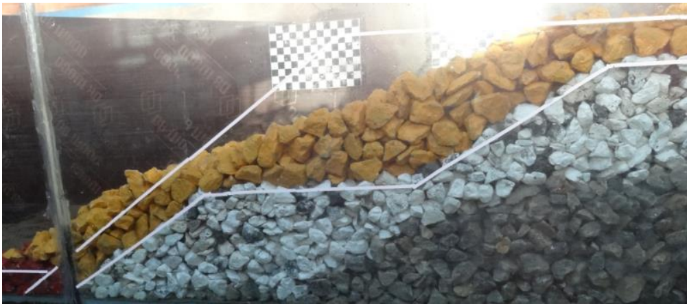
Figure 4.20 View of Section 3 after set 2 (1000 waves)
