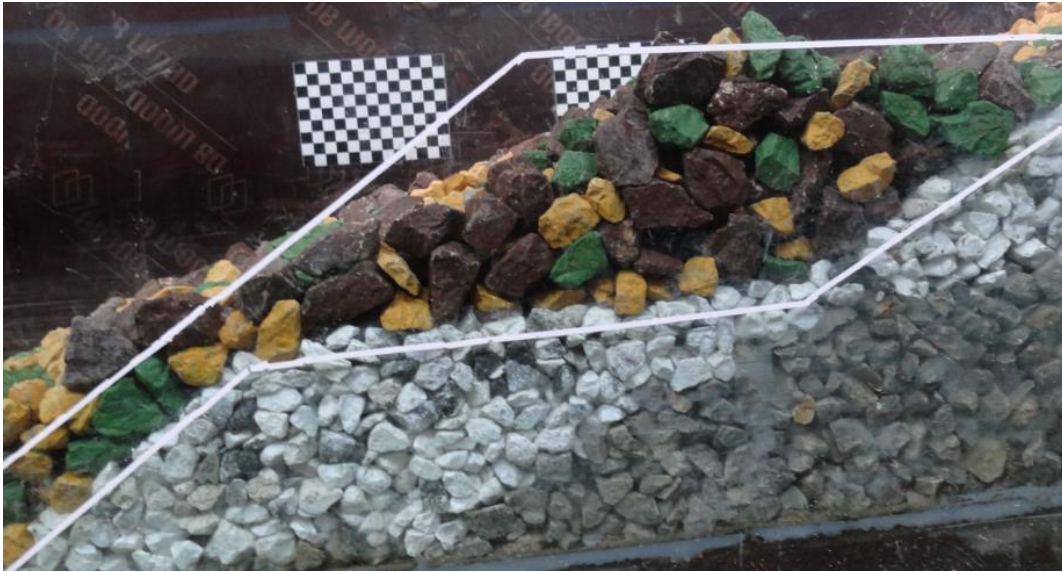
Figure 4.25 View of Section 4 after set 1 (1000 waves)
