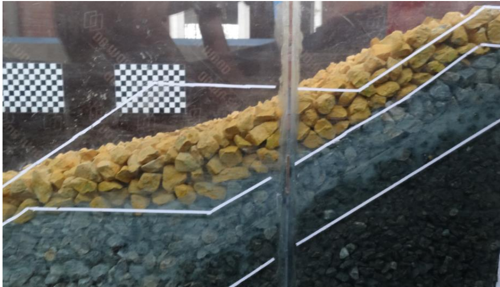
Figure 4.13 View of Section 2 after set 2 (1000 waves)
