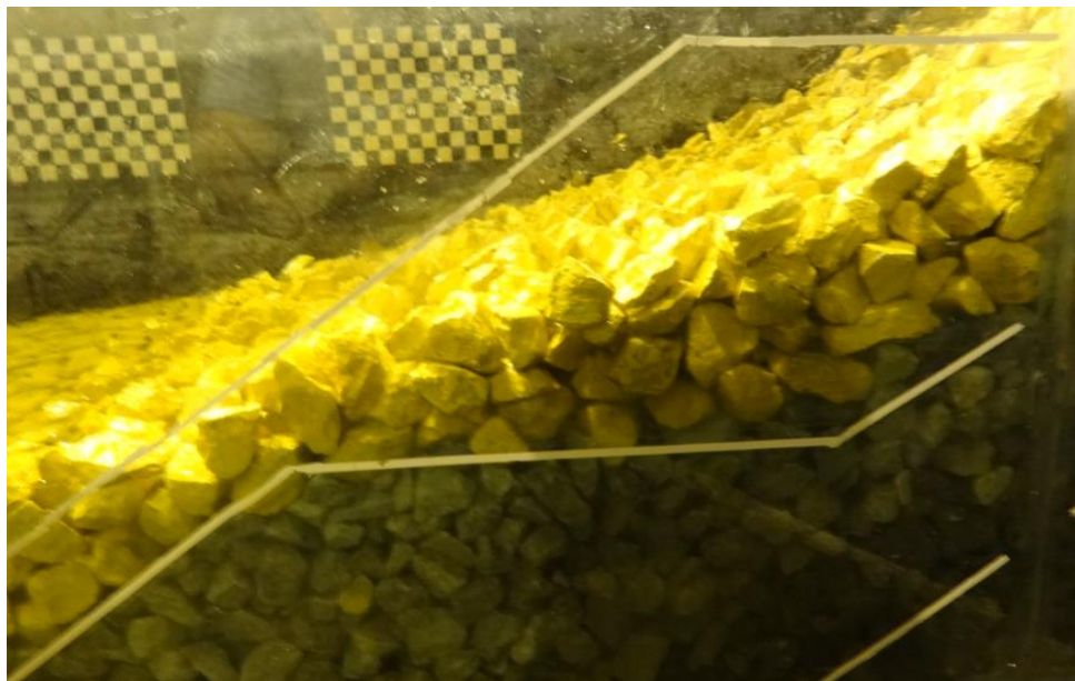
Figure 4.14 View of Section 2 after set 3 (1000 waves)
