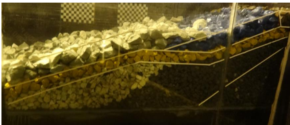
Figure 4.6 View of Section 1 after Set 3 (7000 waves)
