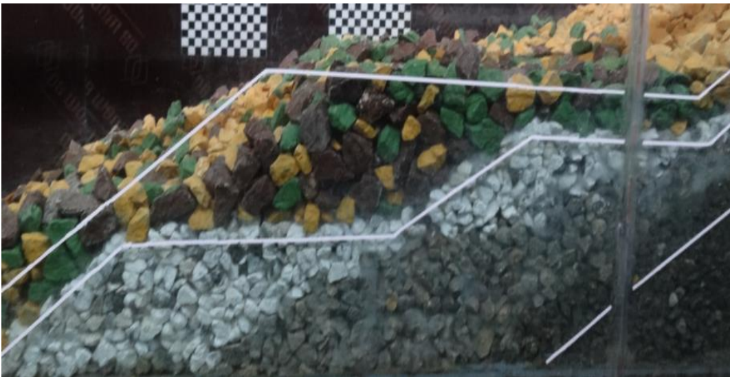
Figure 4.26 View of Section 4 after set 2 (1000 waves)
