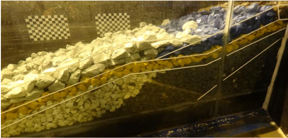
Figure 4.4 View of Section 1 after Set 3 (3000 waves)
