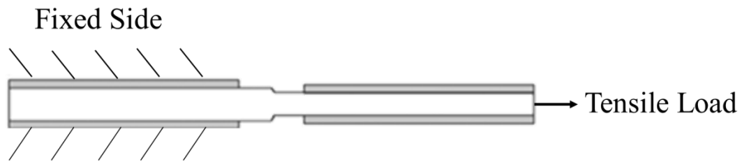
Figure 30. Schematic of the fixed and loaded ends of the tapered laminates
