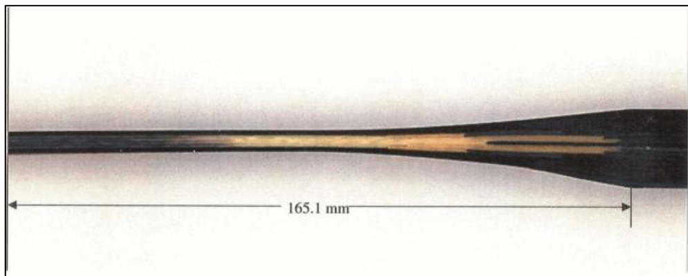
Figure 2. Carbon-glass hybrid flexbeam [1]
