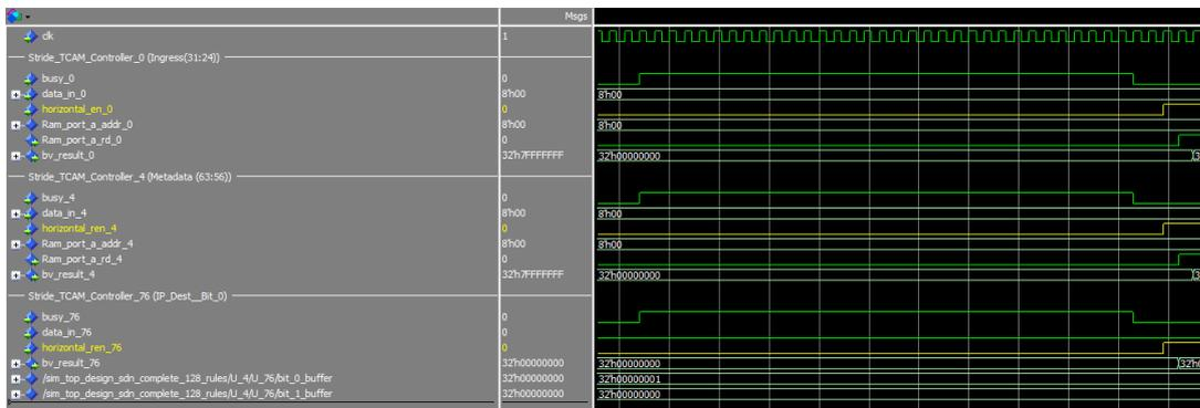
Figure 4.12: Functional simulation of Stride-TCAMs
