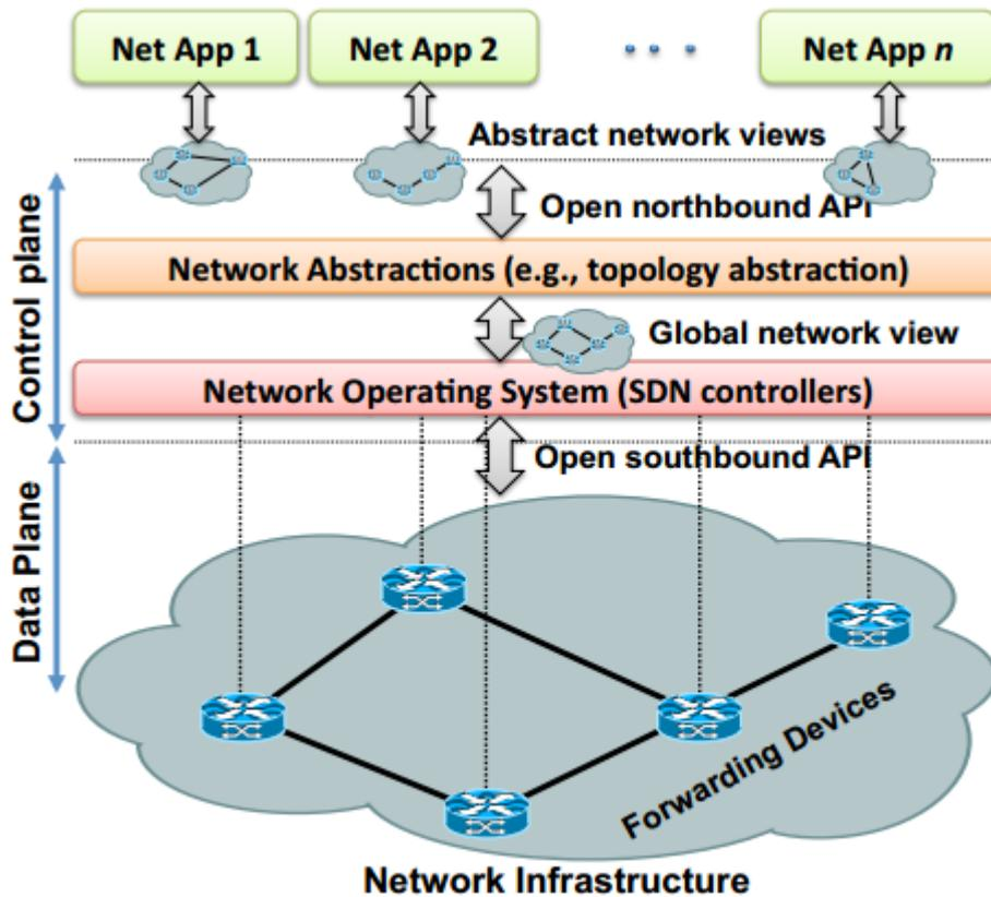
Figure 2.1: Layered architecture of SDN [1]
