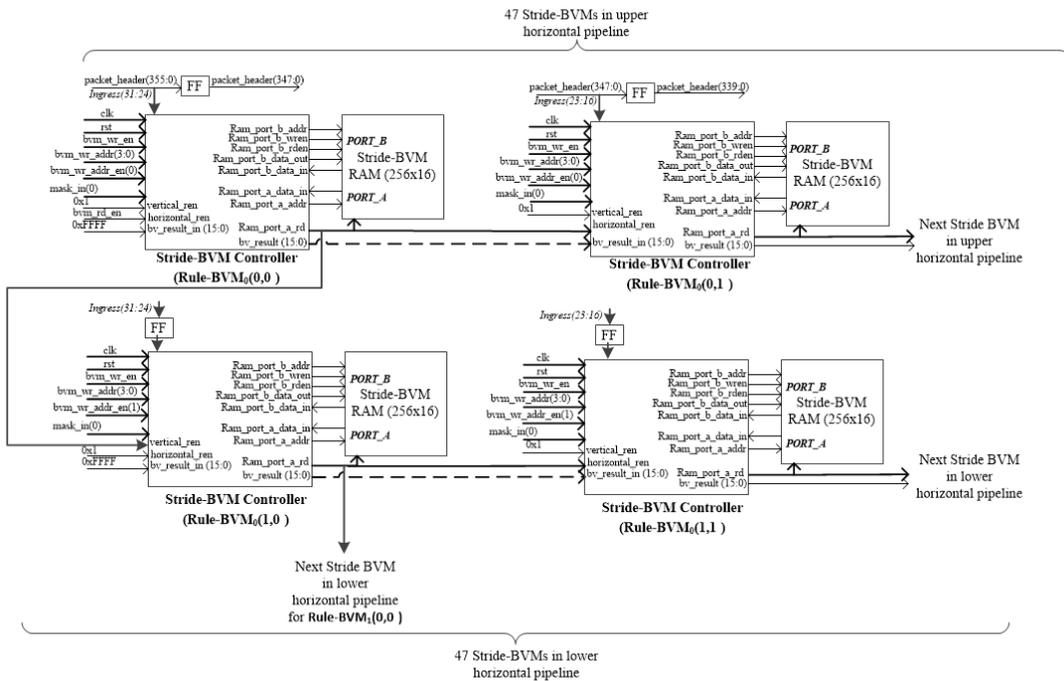
Figure 4.7: Internal architecture of a Rule-BVM for FPGA implementation
