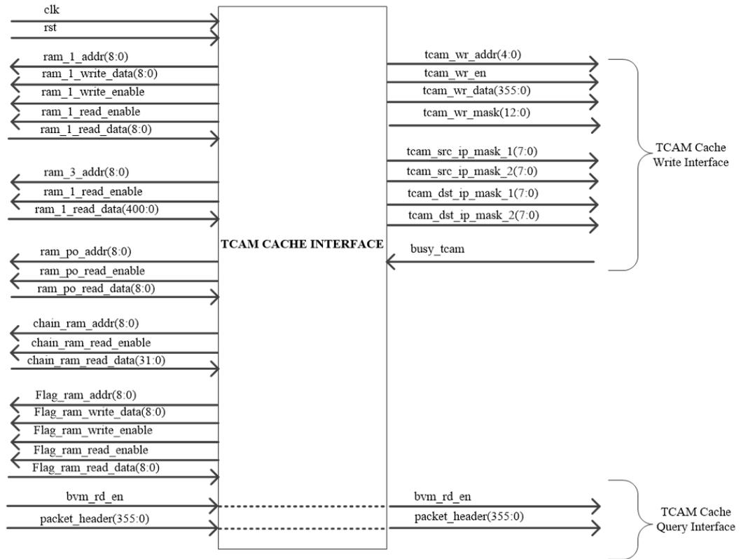
Figure 4.20: Interface diagram of TCAM Cache Interface
