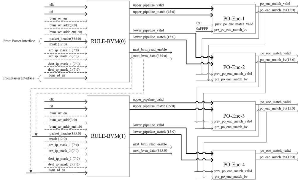
Figure 4.4: Connection diagram of two Rule-BVMs and four Priority Encoders
