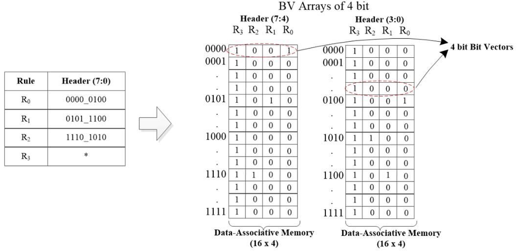
Figure 2.5: Internal structure of data-associative elements
