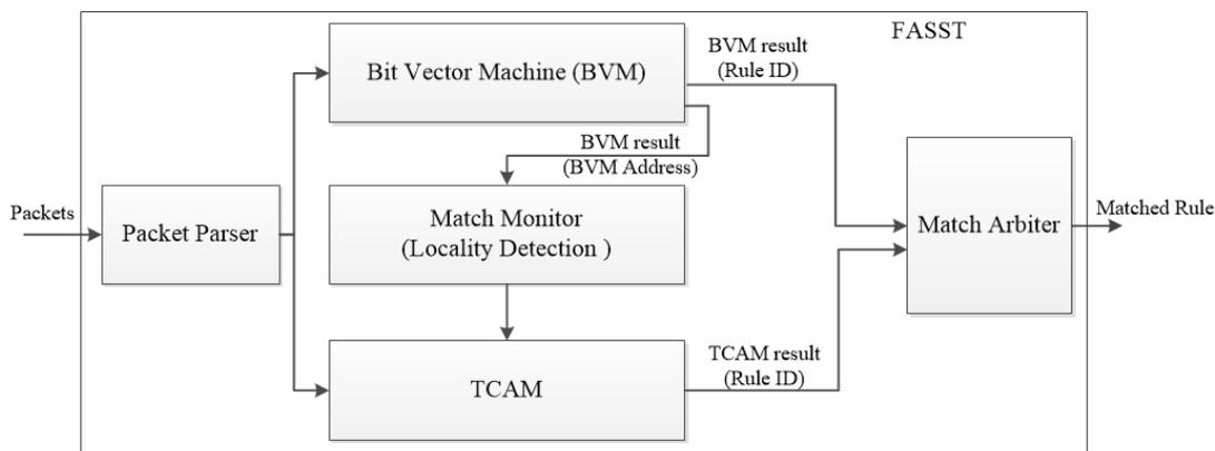
Figure 3.1: Block diagram of FASST architecture
