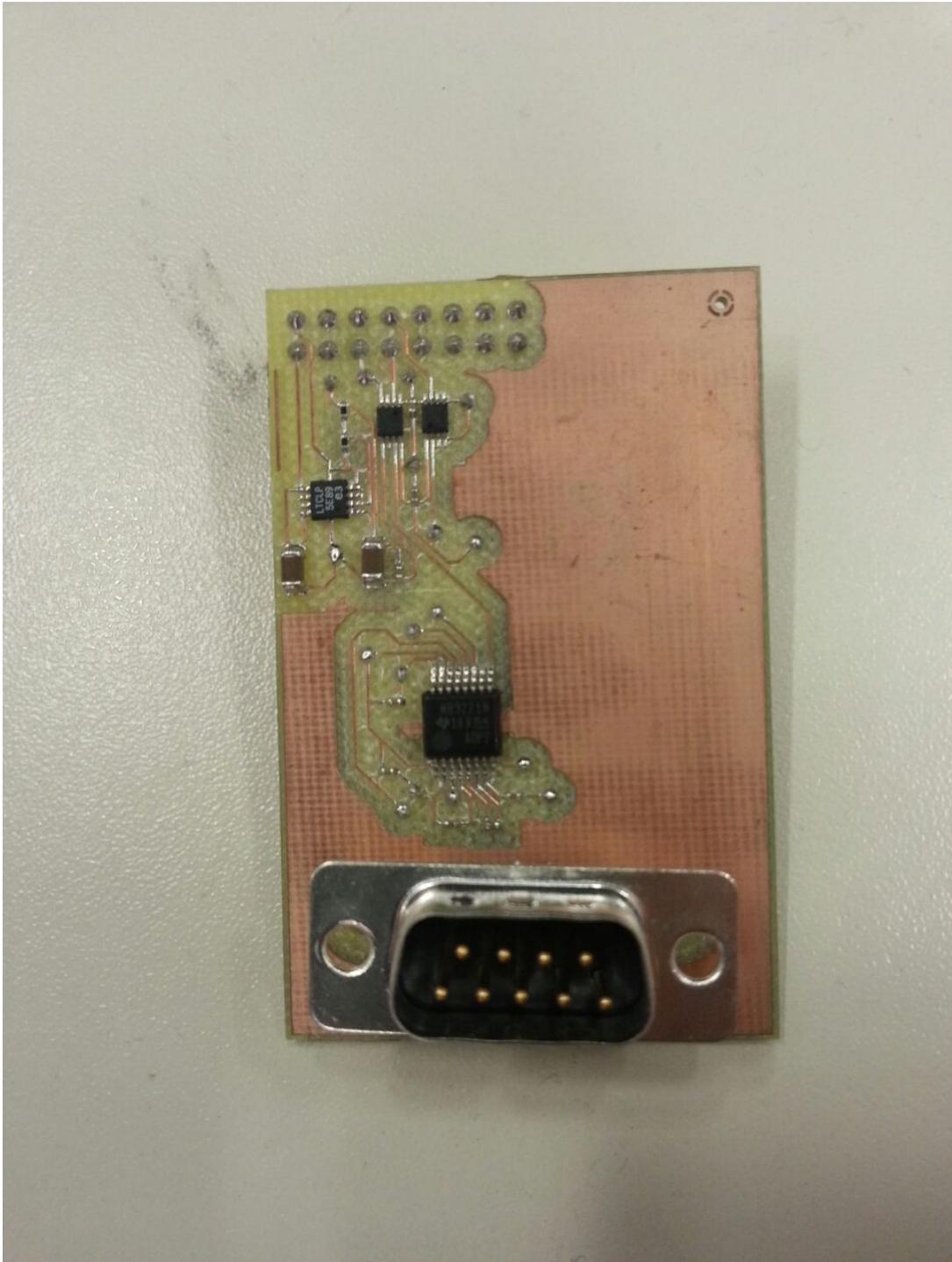
Figure 6.2: RS-232 Add-on interface board
