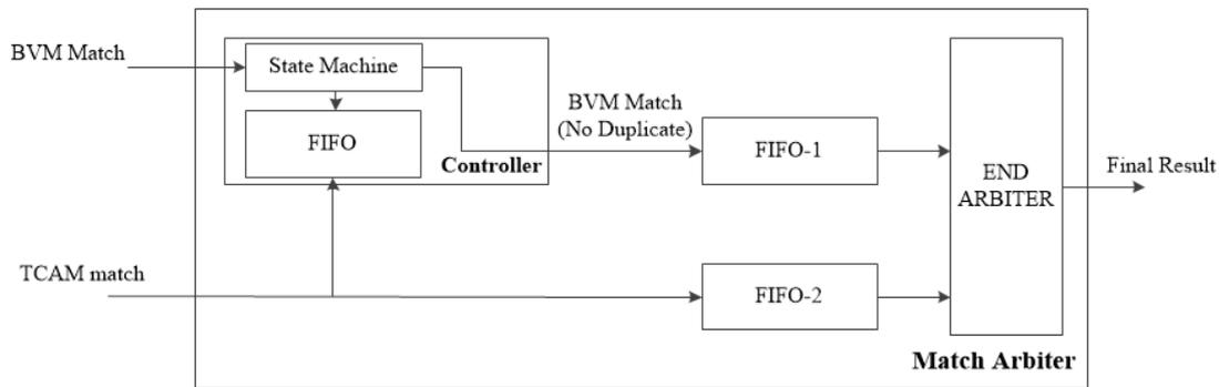
Figure 3.12: Internal block diagram of Match Arbiter Block
