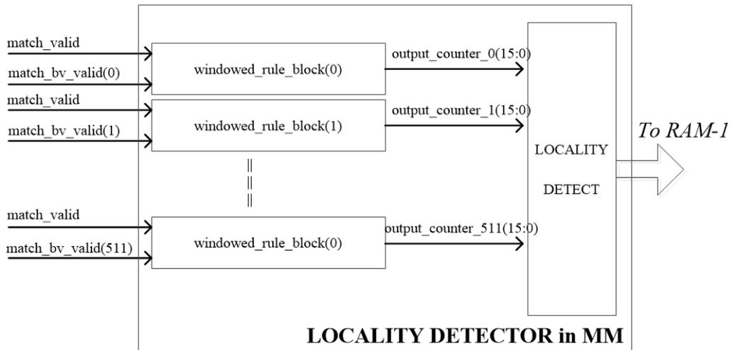
Figure 4.15: Internal architecture of Locality Detector
