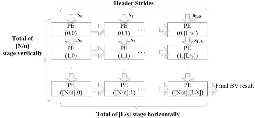
Figure 2.4: Connection of PEs in pipelined BV architecture
