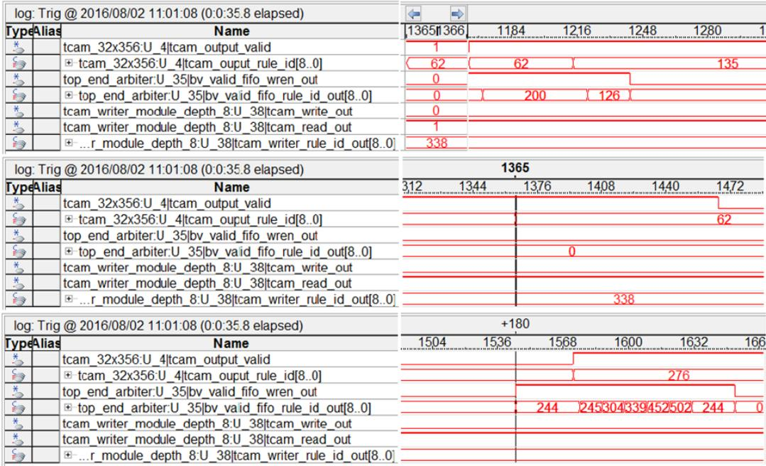
Figure 5.3: TCAM and BVM parallel lookup after first round of locality detection
