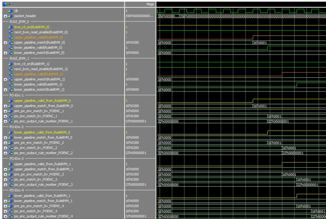
Figure 4.6: Functional simulation of 4 Priority Encoders with vertical pipeline connection
