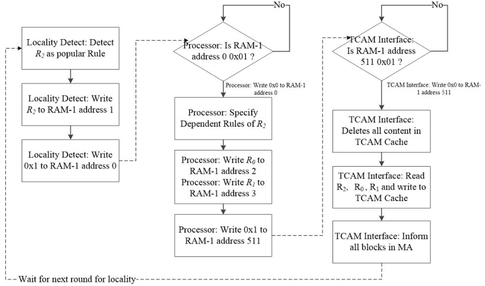
Figure 3.11: Process flow diagram in Match Monitor
