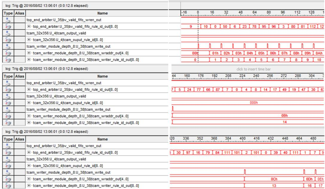
Figure 5.9: TCAM write sequence for popular rule with depth 2
