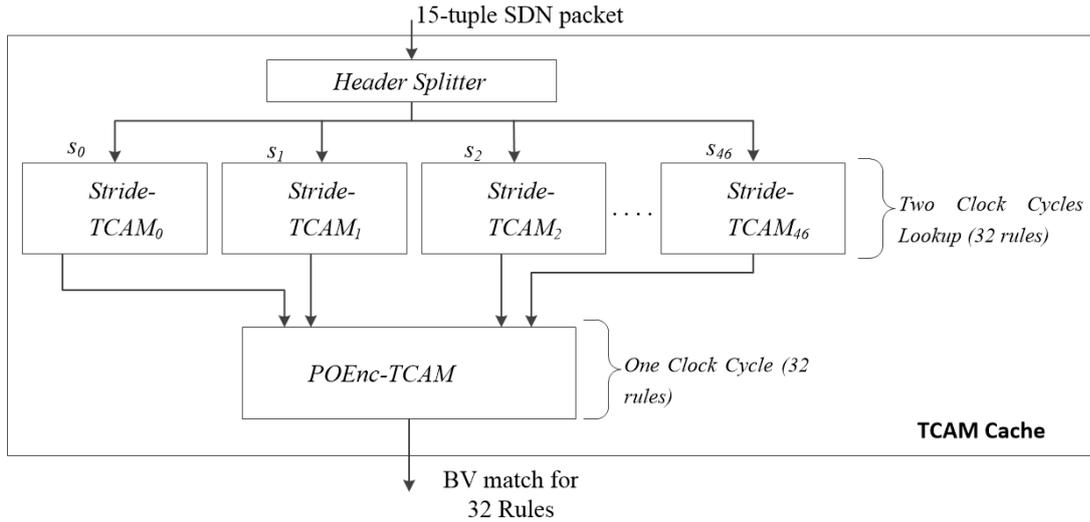
Figure 3.4: Internal parallel architecture of TCAM
