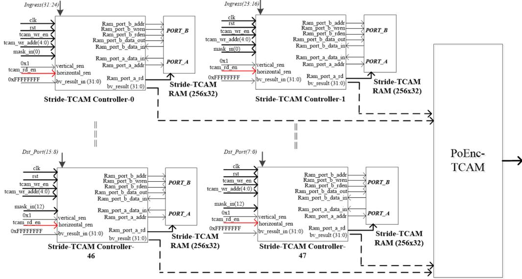
Figure 4.11: Stride-TCAM design in TCAM
