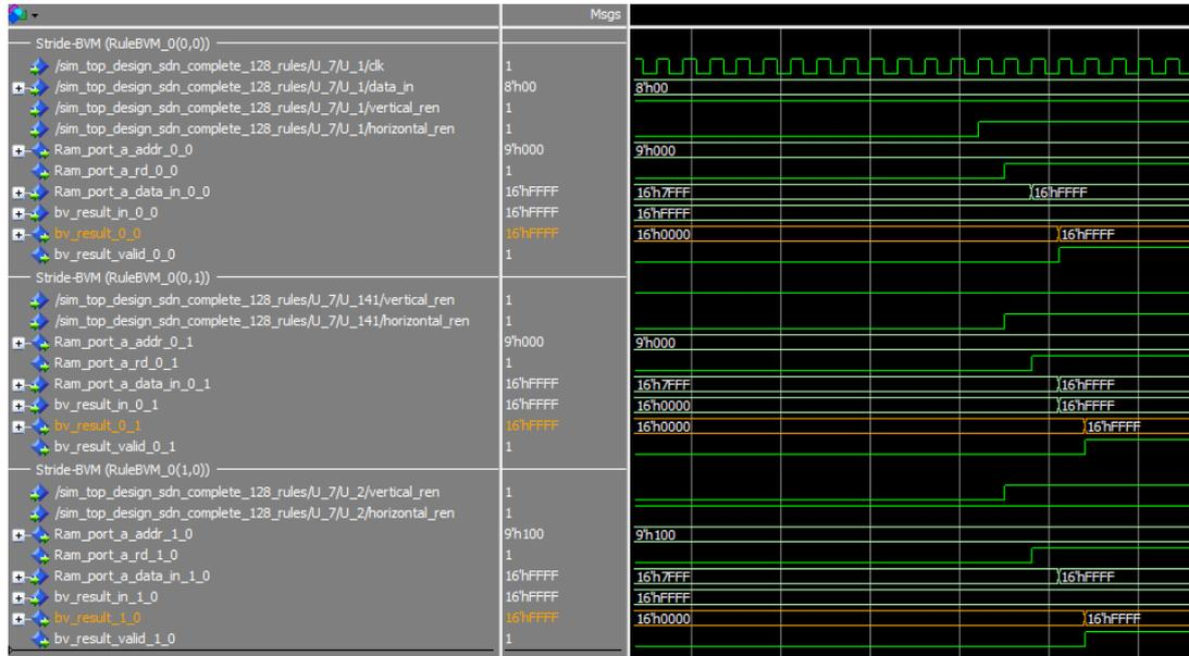
Figure 4.10: Functional simulation of 3 Stride-BVMs with pipeline connection
