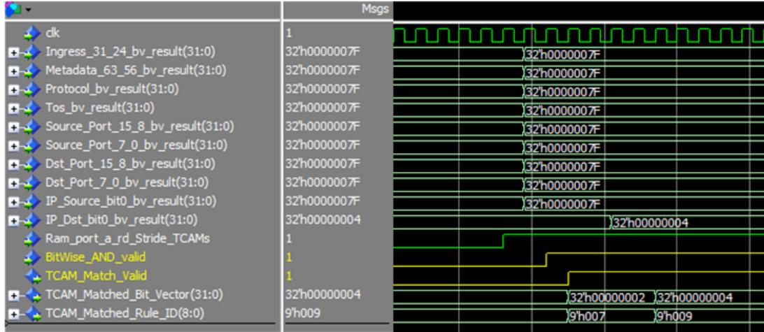
Figure 4.14: Functional simulation of PO-Enc in TCAM
