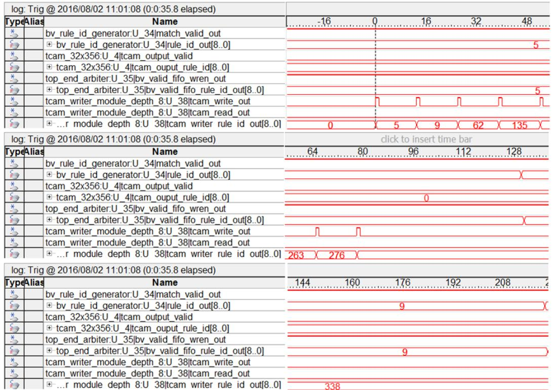
Figure 5.2: First round at locality detection for 7 rules
