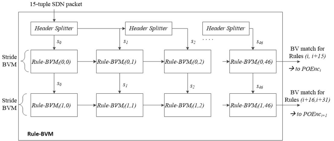
Figure 3.3: Internal pipelined architecture of Rule BVM
