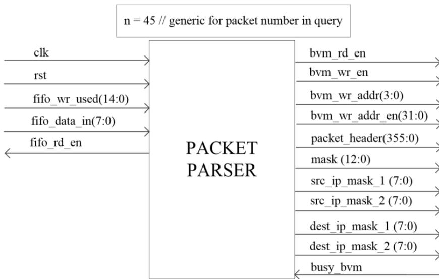
Figure 4.3: Packet Parser Block
