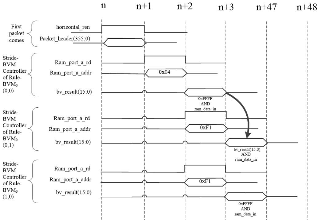
Figure 4.9: Signal level timing diagram for pipeline processing inside Rule-BVM
