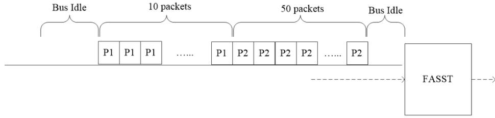
Figure 4.2: Order of incoming packets to FASST for rule query phase
