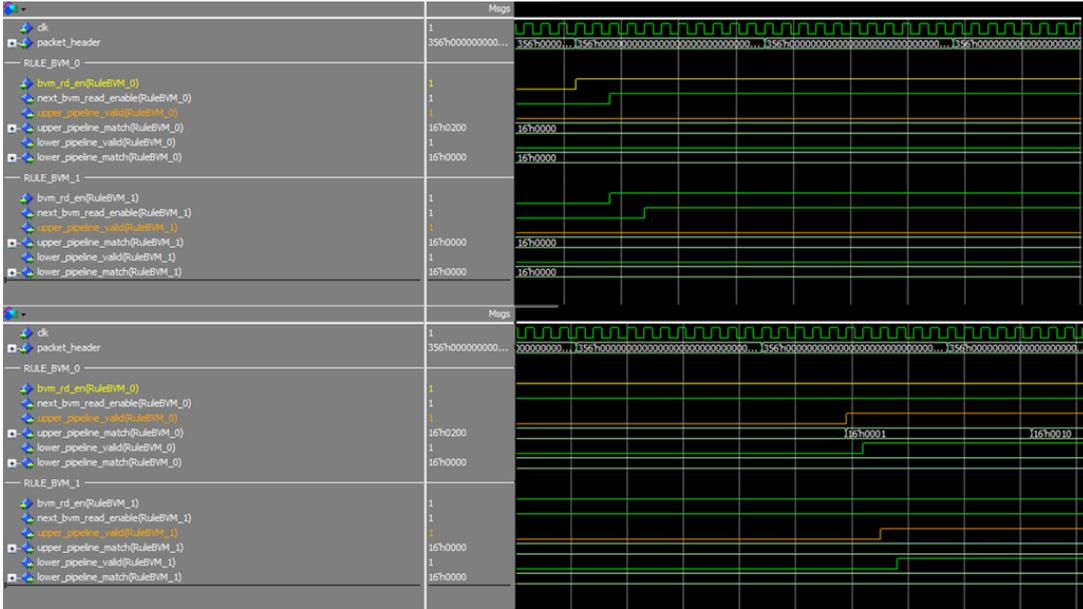
Figure 4.5: Functional simulation of Rule-BVMs for pipeline connection
