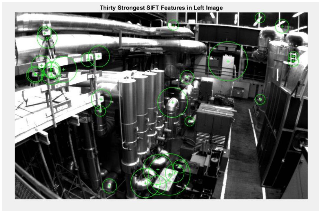
Figure C.3 SIFT features found in the left image
