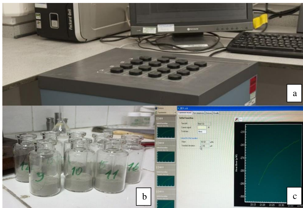
Figure 18. A view of calorimeter cells (a), ampoules (b) and software interface (c)
