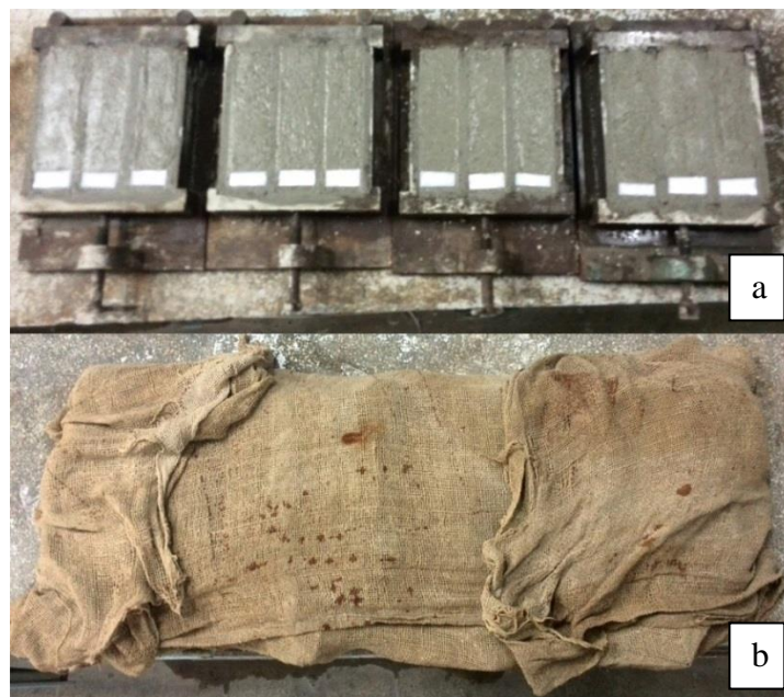
Figure 15. Molded mortar samples(a) and curing technique (b)
