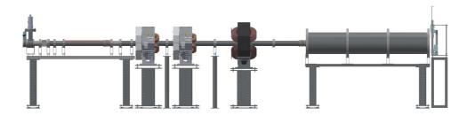
Figure 2.20: The 3-D technical drawing of the final design of METU-DBL includes quadrupole magnets and scattering foils to enlarge the beam size, collimators to reduce the number of particles and a window at the end of the beamline for the beam to exit vacuum. The beam pipes, the vacuum flanges, the support tables of pipes and the target area systems are drawn here in scale.
