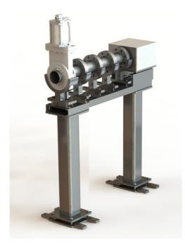
Figure 4.6: The 3D drawing of the energy degradation system for the METU-LEBNA project. It has four titanium foils with 200  $\mu$ m thickness and three helium sections with the length of 10 cm between them.
