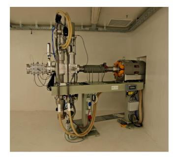
Figure 3.19: The available beam elements in the R&D room. A quadrupole doublet structure extrudes the wall, followed by a solenoid magnet, which will not be used in METU-DBL. A beam viewer and a vacuum dumps follow along the beamline. A 4-jaw collimator is currently the final element, but will be removed when the 5-port switching magnet arrives.
