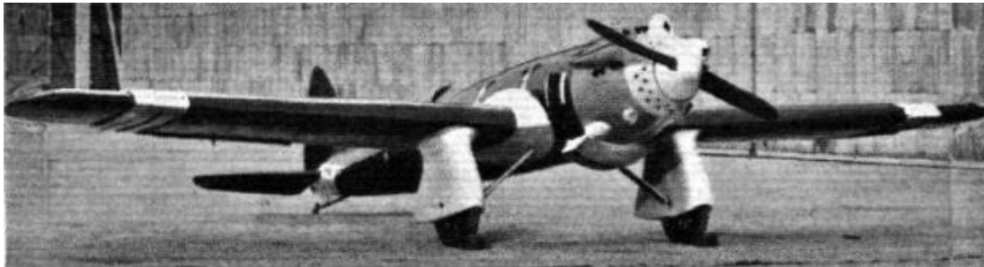
Figure 6: Mak-10 with Wings almost completely Retracted [18]
