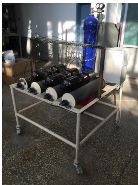
Figure 3.4. Bottle Roll Test Setup
