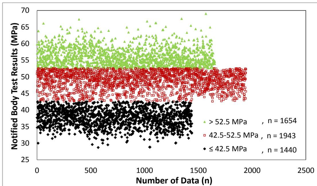
Figure 6: Distribution of Compressive Strength Results according to Strength Intervals
