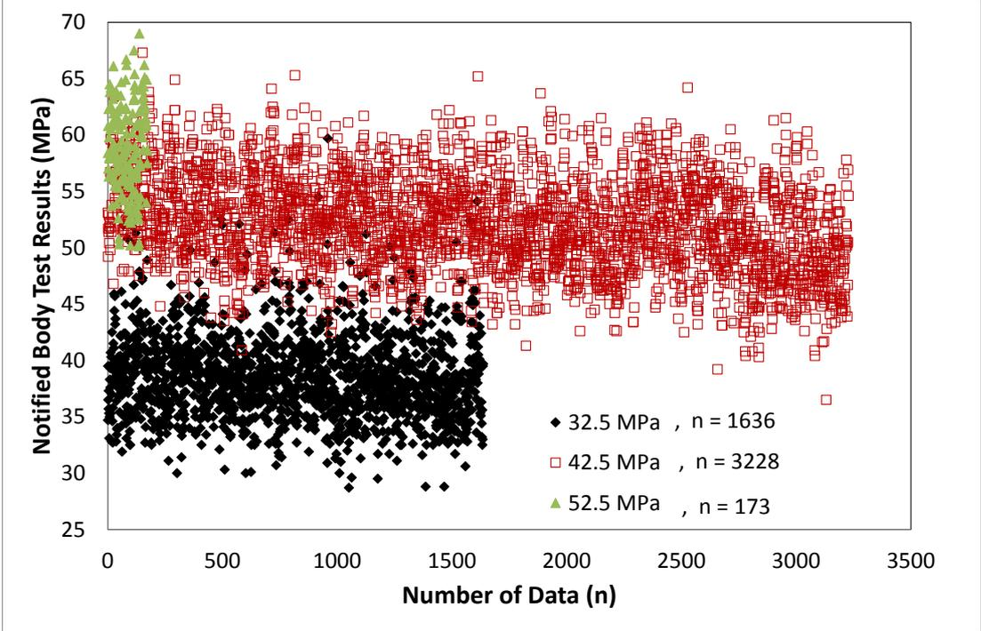
Figure 5: Distribution of Compressive Strength Results according to Strength Classes
