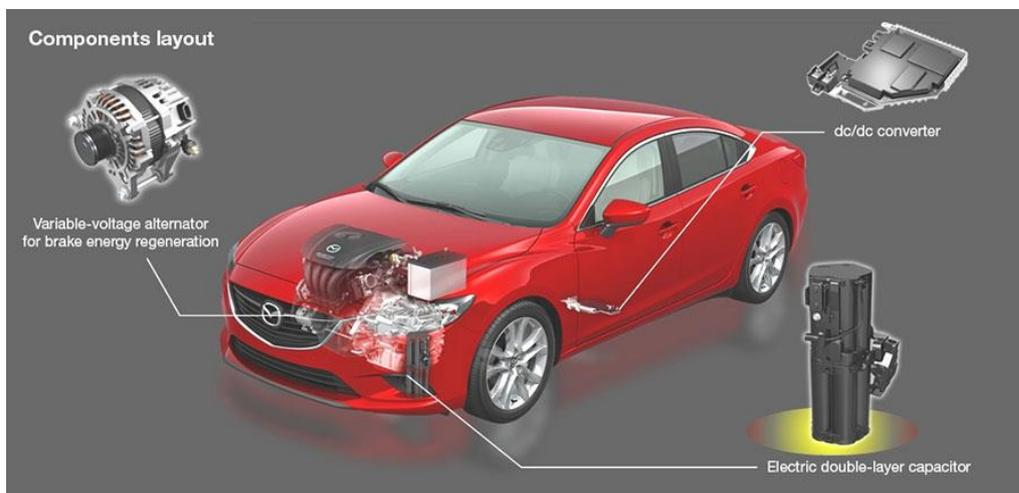
Figure 2. Mazda6 with layout of components in i-ELOOP [10].
