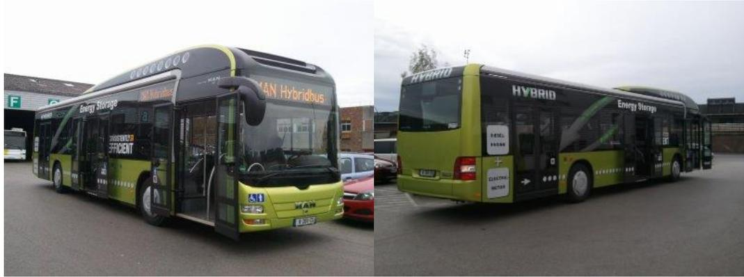
Figure 3. Hybrid bus uses supercapacitors and two 67 kW electric motors [11].
