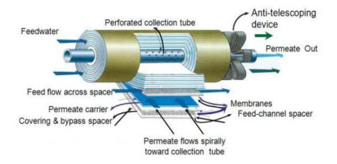
Figure 34: Spiral wounded RO membrane module explanation layer by layer (Buecker, 2016)
