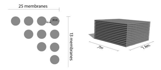
Figure 36: Membrane configuration and dimensions in stack
