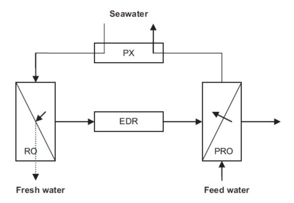
Figure 47:Simple representation of hybrid PRO and RO system (Altaee and Sharif, 2015)
