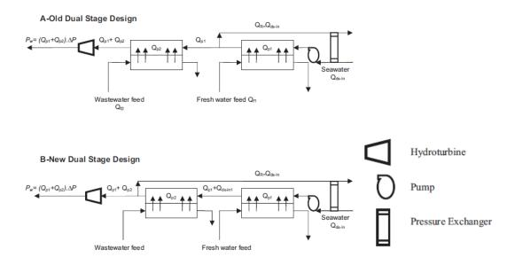
Figure 48 : Comparison of old and new dual stage design for PRO (Altaee and Hilal, 2015)
