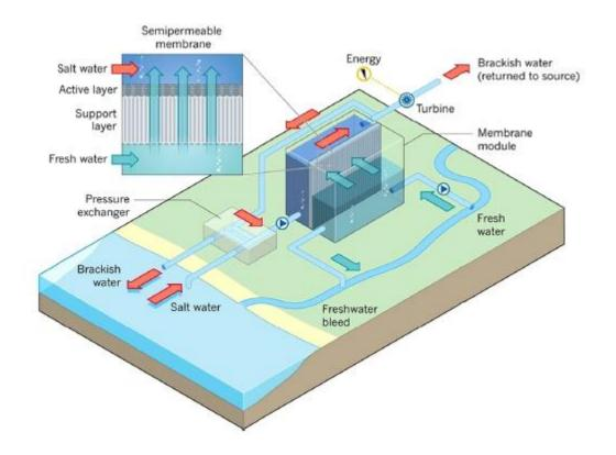
Figure 3:Representation of PRO plant sustained by river water and sea water (Helfer, Lemckert, and Anissimov, 2014).
