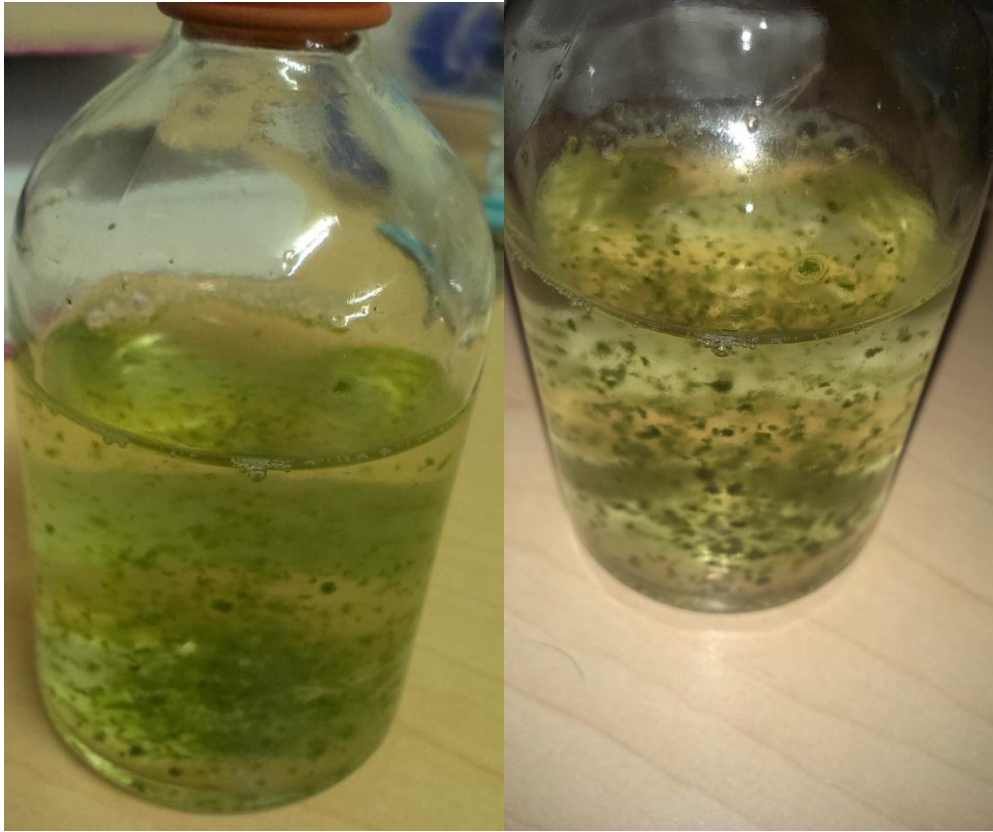
Figure 4-13. Granulation of microalgae in reactors
