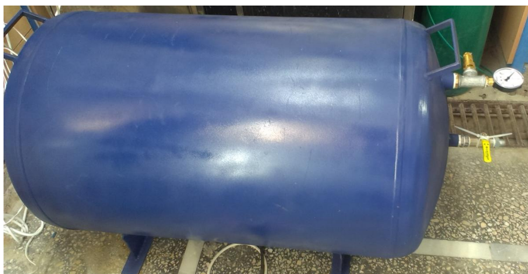
Figure 3-1. 200 liter volume gas cylinder
