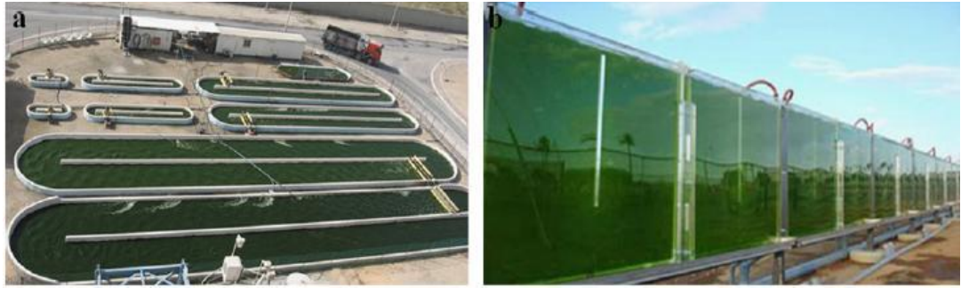
Figure 2-4. Photobioreactors used in growing microalgae: (a) raceway pond, (b) flat-plate type (Bitog et al., 2011)
