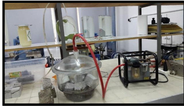
Figure 3.33 The vacuum apparatus used to determine the effective porosity and unit weight of the andesite.
