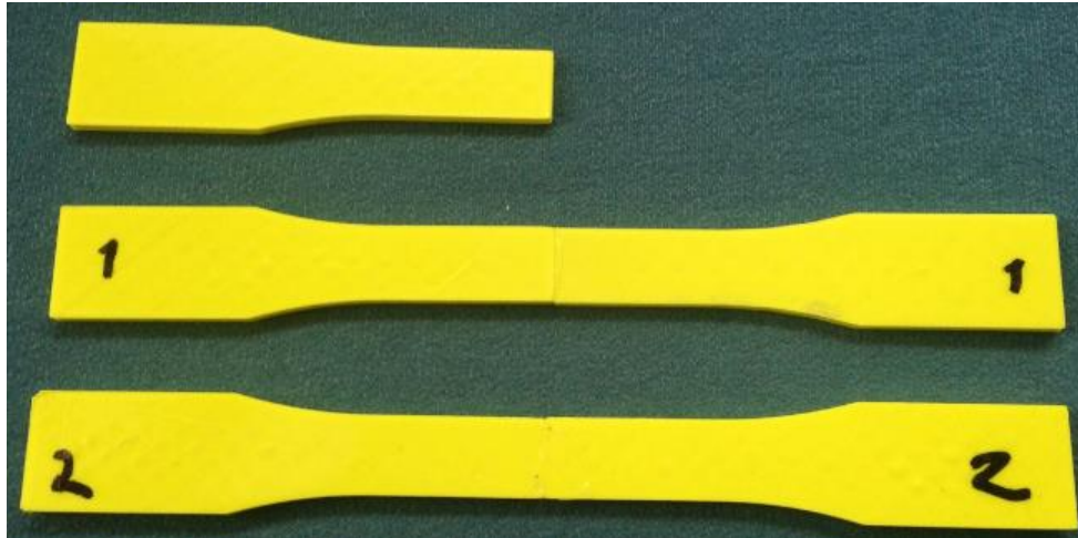
Figure 18. A picture of half specimen and two halves glued together
