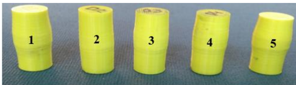
Figure 14. 100% infill cylindrical failed specimens
