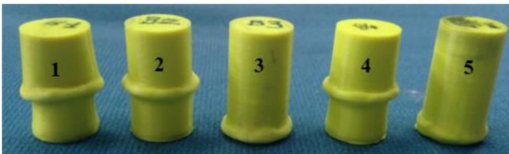
Figure 10. 20% infill cylindrical specimens failed from various regions
