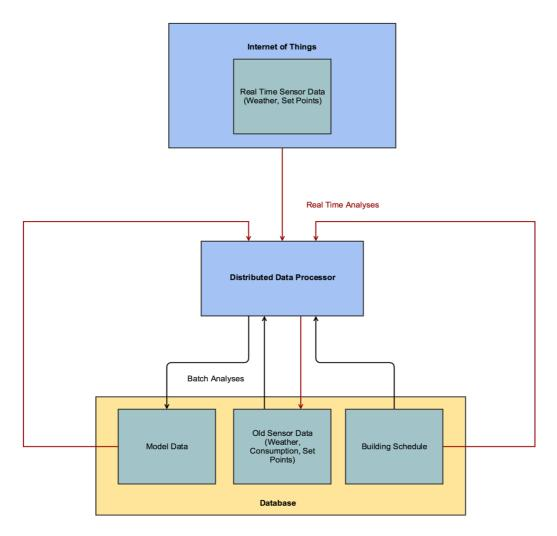
Figure 3: Overall Structure of Big Data Analytics Handling Subsystem
