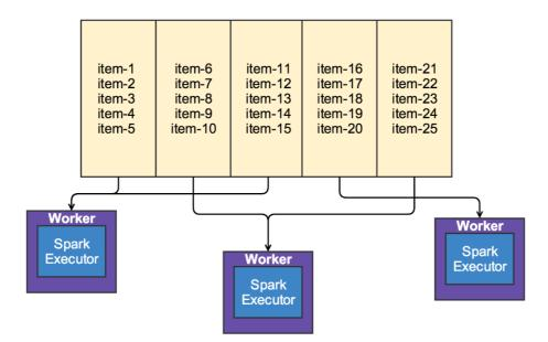
Figure 11: Visualization of RDD Being Partitioned
