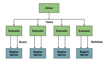
Figure 5: Spark HBase Query Architecture
