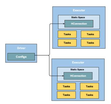
Figure 4: Spark HBase Connection Architecture
