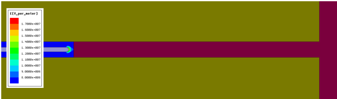
Figure 2-17 Coil with epoxy resin filled in between insulation papers
