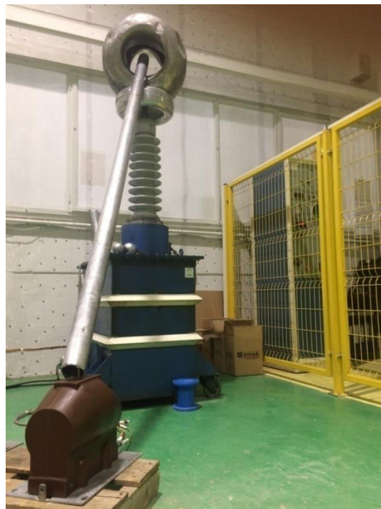
Figure 5-4 Partial discharge test setup
