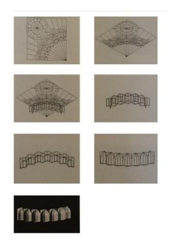
Figure 69. The process of a Muqarnas row transforming into a three-dimensional composition. Source: Necipoglu and Al-Asad. 1996, p.355.
