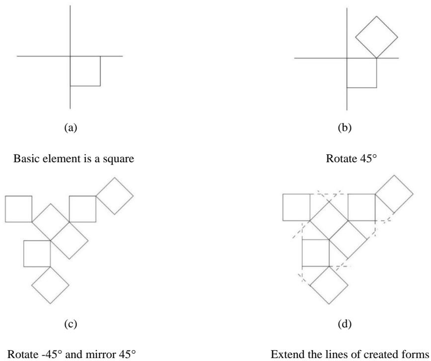
Figure 102. Process of accessing basic module
