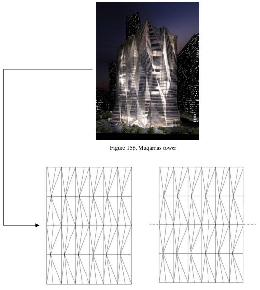
Figure 157. The design of the Muqarnas tower and Decomposition of the pattern to its basic sectors The Patterns are drawn by author
