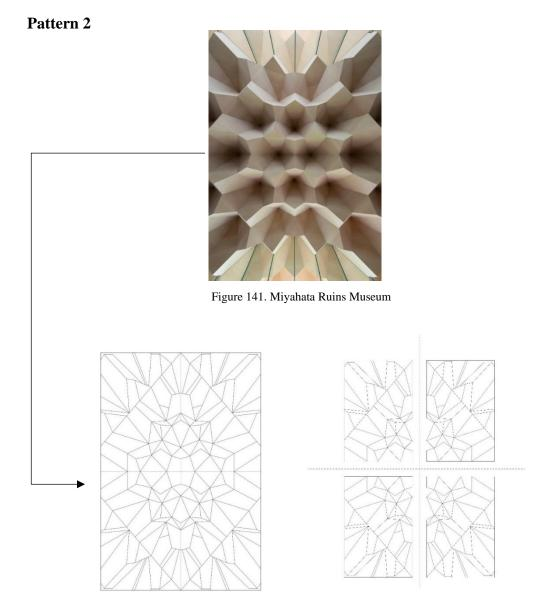
Figure 142. The design of the Muqarnas tower Figure 143. Decomposition of the pattern to its sectors The Patterns are drawn by author
