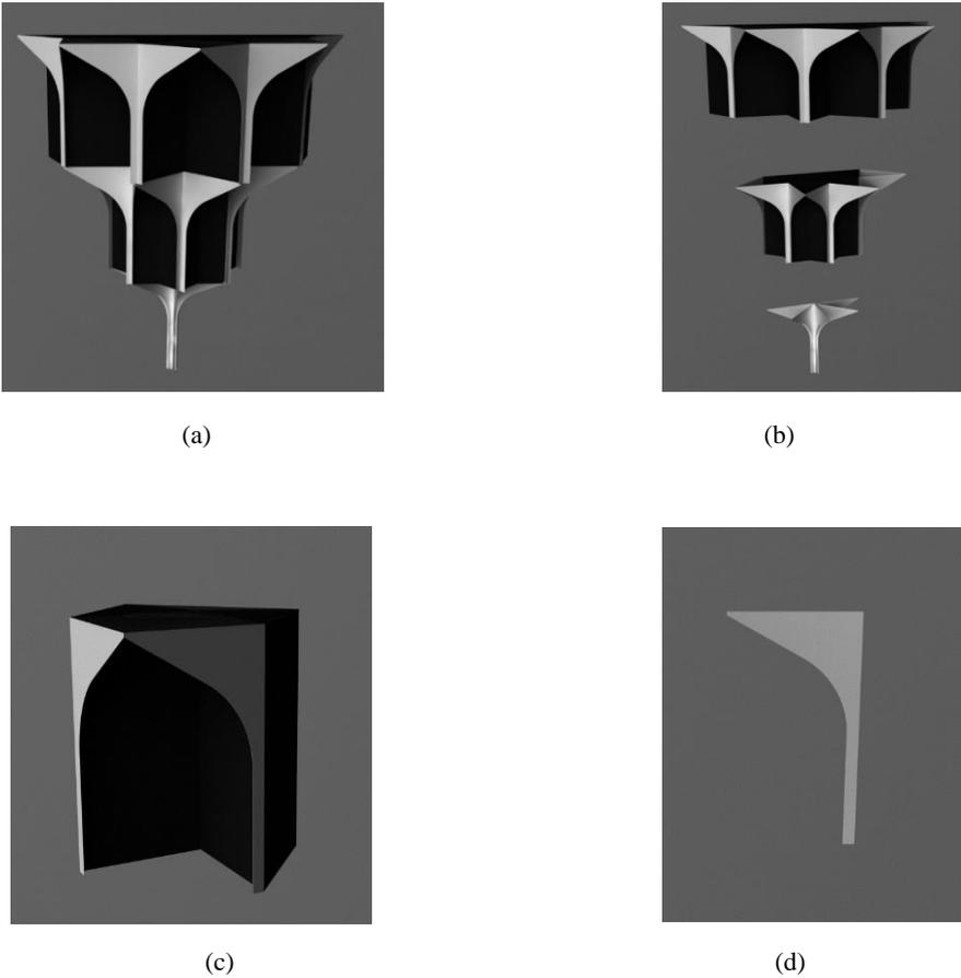
Figure 1. A sample of Muqarnas (a), tiers of Muqarnas (b), a cell (c), an intermediate element (d). (Eric Broug, 2015)
