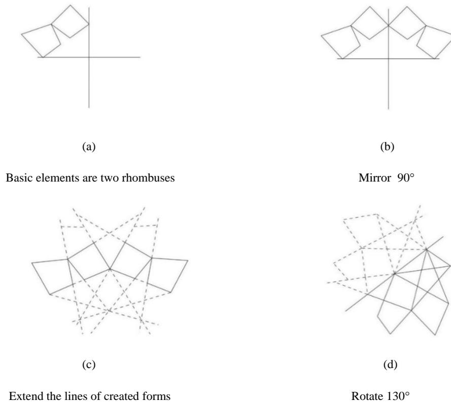
Figure 120. Process of accessing basic module
