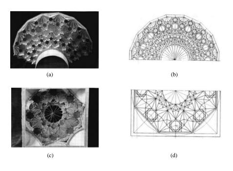
Figure 61. Ustad Shirin Muradov's sketches of stalactites and their spatial treatment in scale models made of paper. Muqarnas model (a), Muqarnas sketch (b), Muqarnas model (c), Muqarnas sketch (d).
