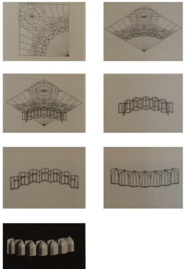
Figure 69. The process of a Muqarnas row transforming into a three-dimensional composition.
