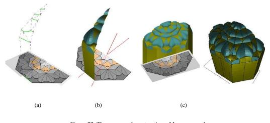
Figure 72. The process of constructing a Muqarnas vault Binding the layers (a), a completed motif (b), Figure Completed Muqarnas vault (c) Source: Hamekasi, Samavati and Nasri. 2011, p.134.
