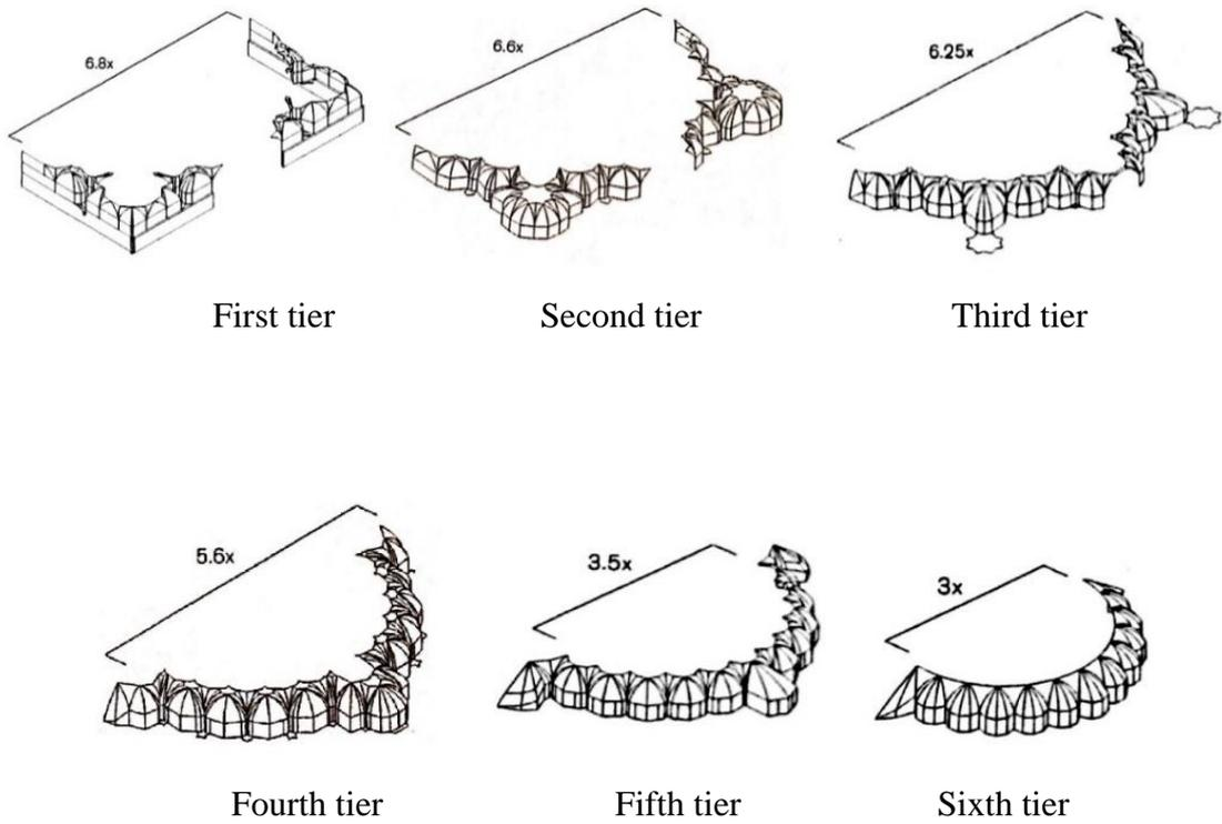
Figure 59. Process for constructing a Muqarnas composition
