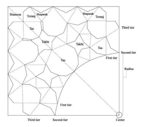
Figure 44. Two-dimensional plane projection of a Muqarnas composition (Web 36) Figure is redrawn by author
