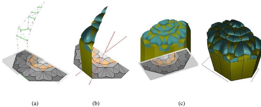
Figure 72. The process of constructing a Muqarnas vault
