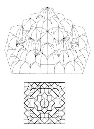
Figure 65. Reconstruction of the Muqarnas of the vault of Takhti-suleyman Source: Yaghan. 2000, p.80.
