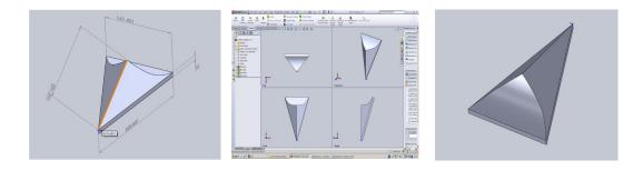
Figure 75. Muqarnas element design process Source: Alkandari. 2011, p.319.
