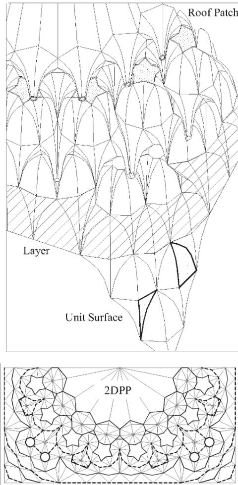
Figure 57. The basic parts of the Muqarnas (Web 37)
