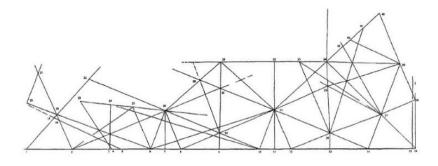
Figure 60. Construction of the Central Muqarnas vault Source: Ghazarian and Ousterhout. 2001, p.148.
