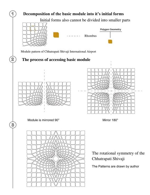
The rotational symmetry of the pattern shows that, exactly like Azadi tower's pattern, this pattern was created as a whole initially with CAD systems. According to the generative aspects of its basic sector, it is impossible to achieve this pattern like traditional ways from part to whole.
