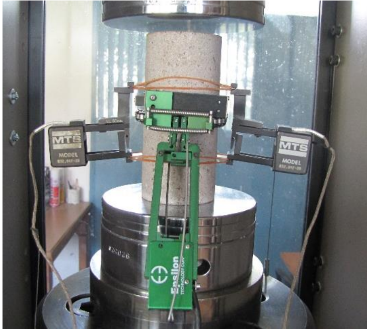
Figure 4. 1 A typical andesite specimen ready for the deformability test with axial and lateral extensometers
