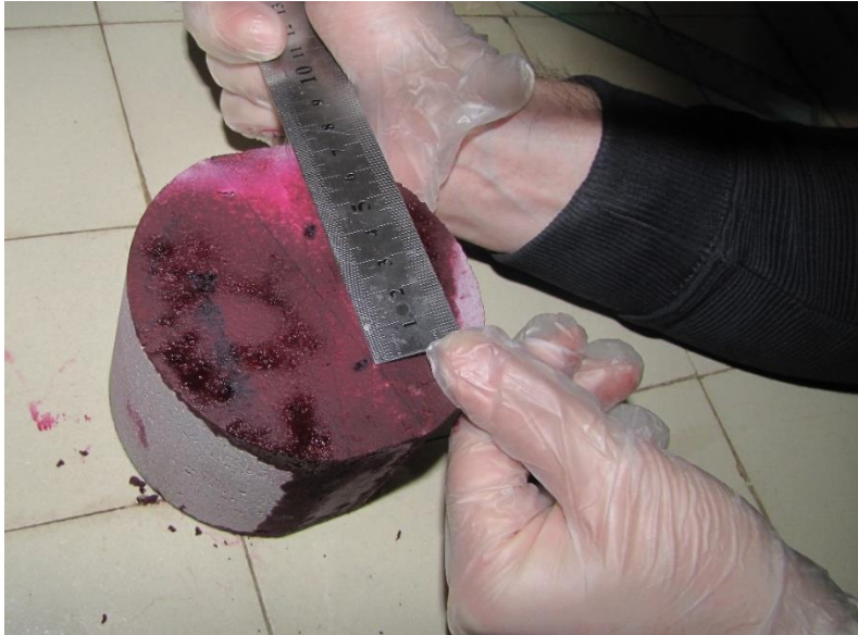
Figure 4. 17 Experimental critical crack length measurement by ruler after fracturing and dye penetrant spray application
