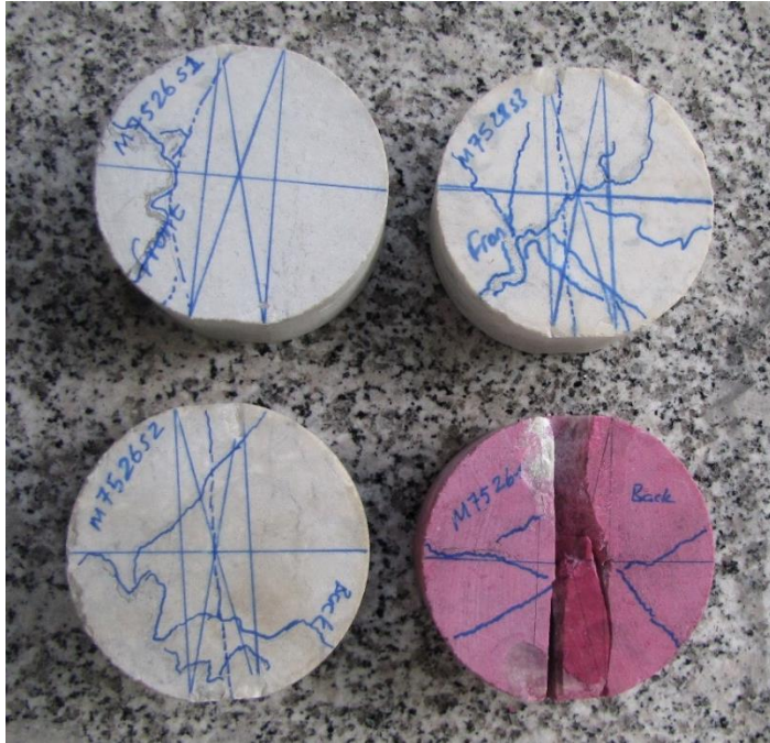
Figure C . 2 Back and front views of marbles having 75 mm in diameter with discontinuities parallel to loading direction (not considered in calculations since it is possible to influence the loading conditions.)
