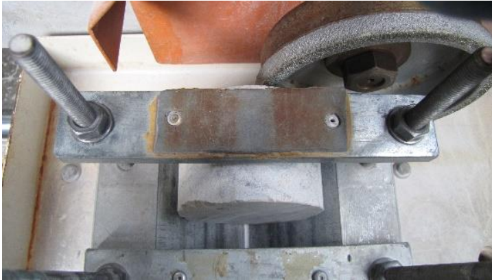
Figure 4. 8 Adjustment of thickness in diametral position
