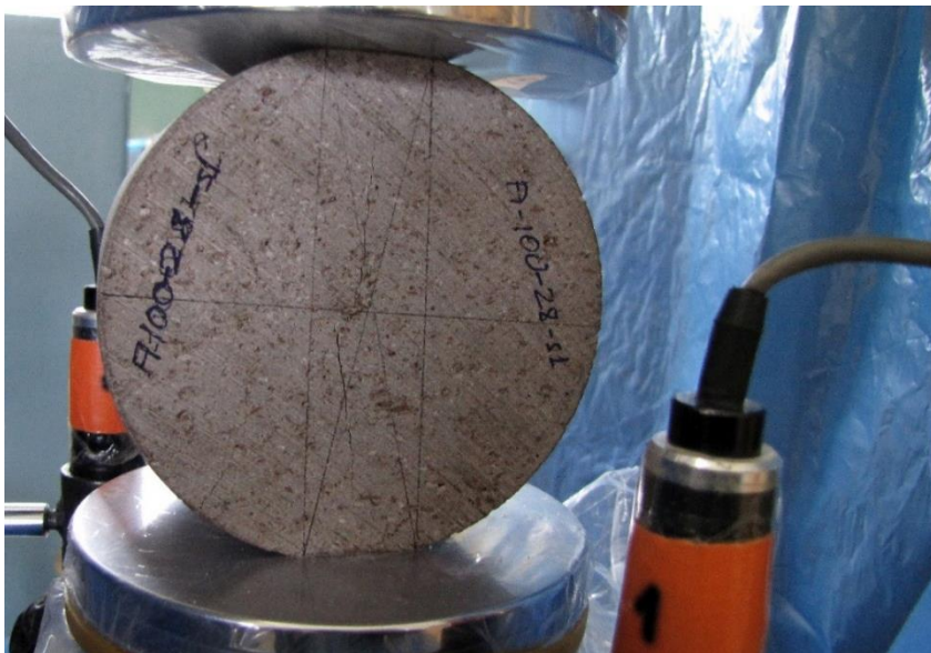
Figure 4. 15 Experimental critical crack length formation at minimum load
