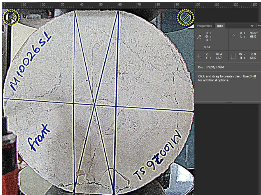
Figure D. 12 Front view of M10027s1 specimen with 2a_{ce} = 66.5 mm
