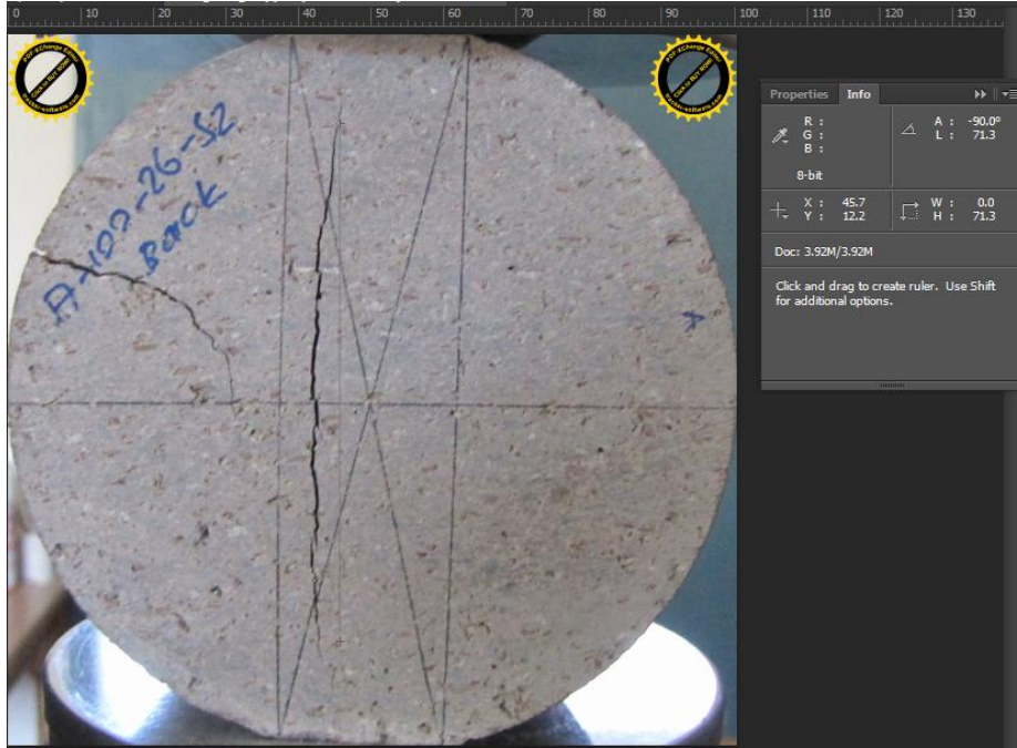
Figure D. 6 Back view of A10026s2 specimen with 2a_{ce}=71.3 mm
