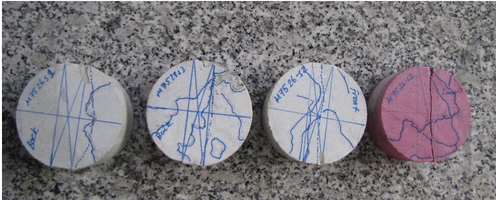
Figure 4. 13 Typical 75 mm diameter marbles with discontinuities parallel to loading direction
