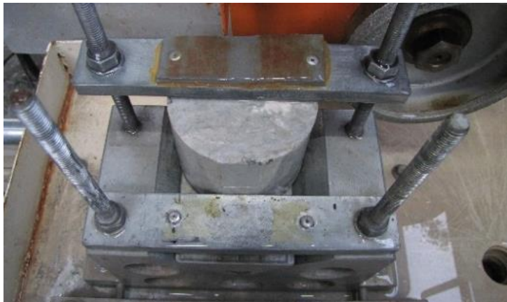
Figure 4. 10 Constructing parallel flat surfaces with a horizontal set (axially positioned)
