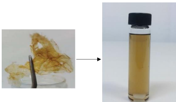
Figure 4.1.2 Obtained GO in the bulk form (left) and an aqueous dispersion of GO (right).
