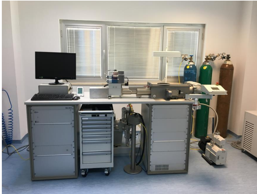
Figure 18 TA-BAEHR DIL805T deformation dilatometer
