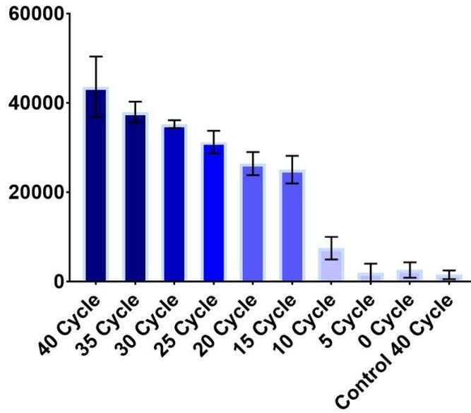
**Figure 3.32:** The graph of SIs on LFAs with Probe-1 capped SiNPs, onto which, target amplicon (20 ng input DNA was added in 50  $\mu$ L PCR solution) with various number of cycle (40, 35, 30, 25, 20, 15, 10, 5, 0) and control amplicon (40 cycle) were applied separately. Until 10 cycle, LFAs could response complementary targets. LoD was determined as 15 Cycle.
