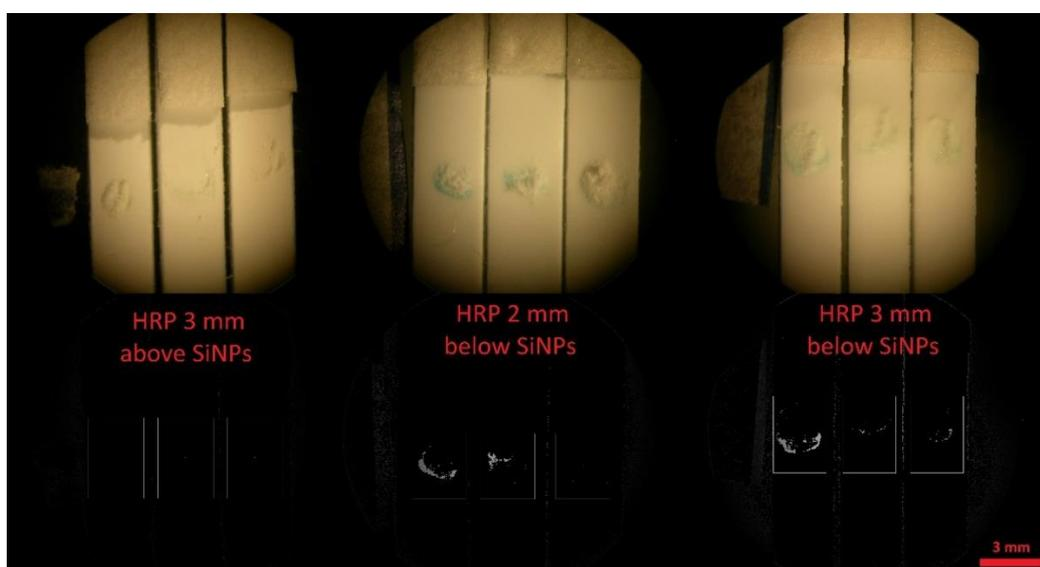
**Figure 3.19:** The image of LFAs in which HRP were located on different positions: 3 mm above SiNPs, 2 mm below SiNPs and 3 mm below SiNPs. ([TMB] = 5 mM, 1% H<sub>2</sub>O<sub>2</sub>, 0.5 mg/mL of HRP and 37°C)
