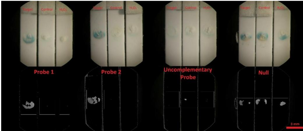
**Figure 3.22:** The image of LFAs including SiNPs capped with Probe-1, Probe-2, Uncomplementary Probe and uncapped. ([TMB] = 5 mM, 1% H<sub>2</sub>O<sub>2</sub>, 0.5 mg/mL of HRP and 37°C)
