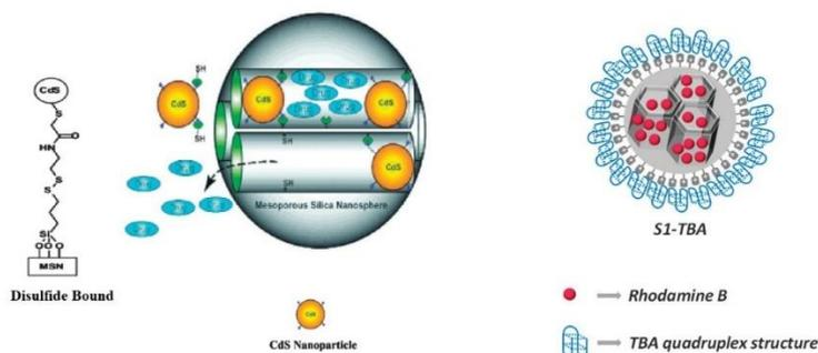
**Figure 1.3:** Cadmium QDs (CdS) are packed into SiNPs (MCM-41) so that toxicity of cadmium can be prevented. CdS is immobilized on MCM-41 via disulfide bridge (S. H. Wu, C. Y. Mou and H. P. Lin, 2013). Rhodamine B are packed in SiNPs (MCM-41) and functionalization is obtained via electrostatic interaction between aptamer and silane coated surface (Mar Oroval et al., 2013).
