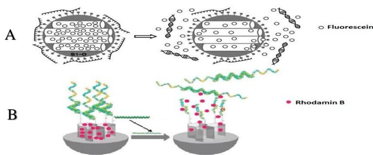
**Figure 1.6:** A. Electrochemical binding of probes (E. Climent et al., 2010) B. Covalent binding of probes (Luis Pascual et al., 2014)
