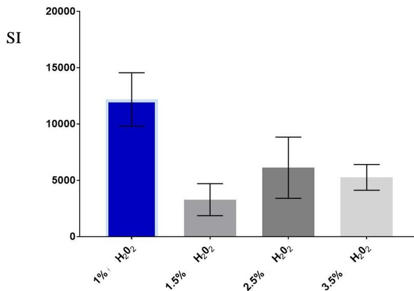
**Figure 3.4:** Signal Intensities (SIs) for various concentration of  $H_2O_2$ : 1%, 1.5%, 2.5% and 3.5%  $H_2O_2$ . Even though there is not any meaningful difference between concentrations of  $H_2O_2$  (ANOVA,  $P > 0.05$ ); 1%  $H_2O_2$ , blue in graph, gives highest SI.
