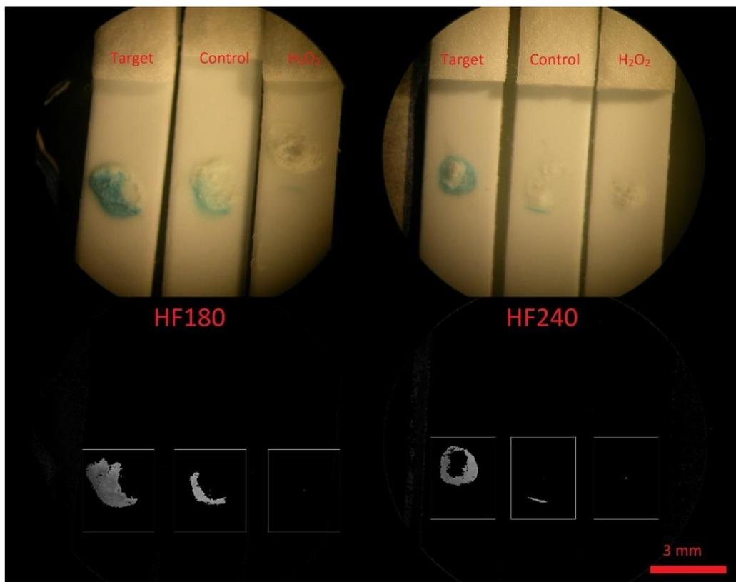
**Figure 3.17:** The images of LFAs with different nitrocellulose membranes: HF180 and HF240. ([TMB] = 5 mM, 1% H<sub>2</sub>O<sub>2</sub>, 0.5 mg/mL of HRP and 37°C)
