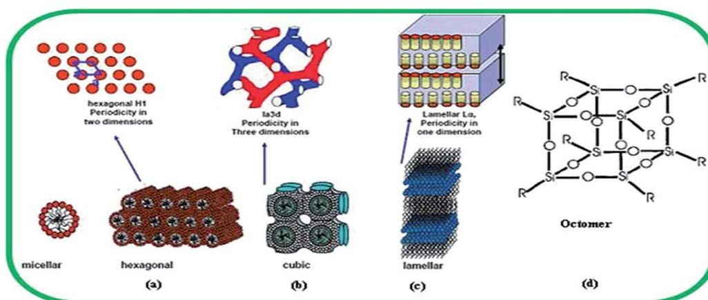
**Figure 1.2:** Some structures of Mesoporous Silica Nanoparticles. A. MCM-41 with hexagonal dimension. B. MCM-48 with cubic dimension C. MCM-50 with lamellar dimension. D. Octomer dimension
