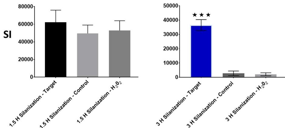
**Figure 3.14:** The graph of SI was obtained from SiNPs which had been prepared with 1.5 hours and 3 hours silanization. Target caused significantly high SI on LFAs, prepared with 3 hours silanization (one-way ANOVA, Tukey HSD test,  $P < 0.001$ ,  $n=3$ ), while 1.5 hours silanization could not properly generate SI on LFAs (one-way ANOVA,  $P > 0.05$ ,  $n=3$ ).
