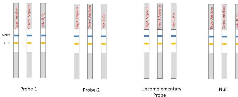
**Figure 2.2:** Experimental scheme of colorimetric response of complementary oligonucleotide (Probe-1 and Probe-2) capped SiNPs, Uncomplimentary Probe capped SiNPs and Null SiNPs on LFAs
