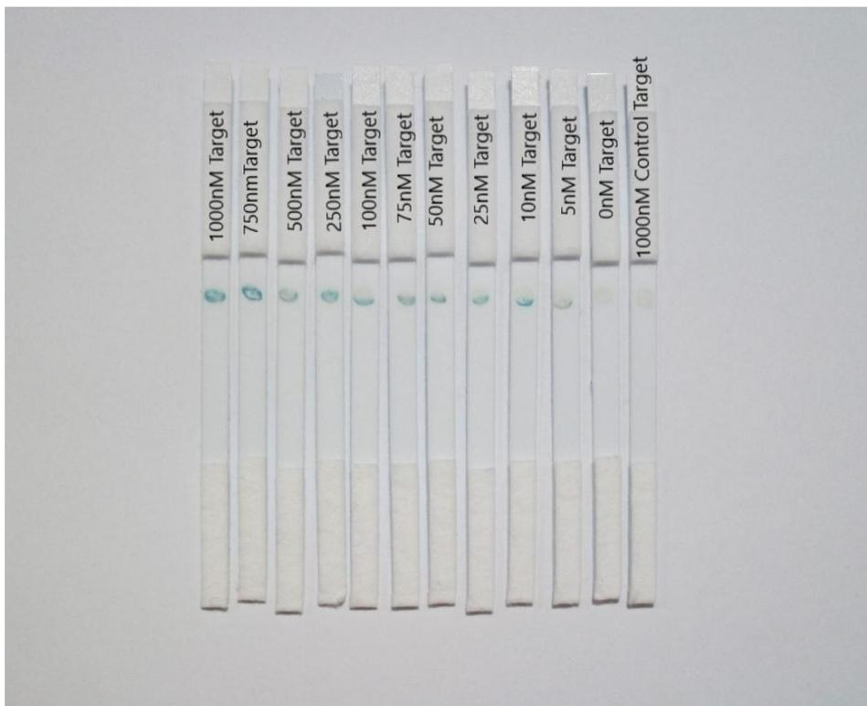
**Figure 3.28:** The overall image of LFAs, including Probe-2 capped SiNPs, onto which, gradual concentration of synthetic complementary Target-2 (1000 nM, 750 nM, 500 nM, 250 nM, 100 nM, 75 nM, 25 nM, 10 nM, 5 nM and 0 nM) and 1000 nM of uncomplementary Control Target. ([TMB] = 5 mM, 1% H<sub>2</sub>O<sub>2</sub>, 0.5 mg/mL of HRP and 37°C)
