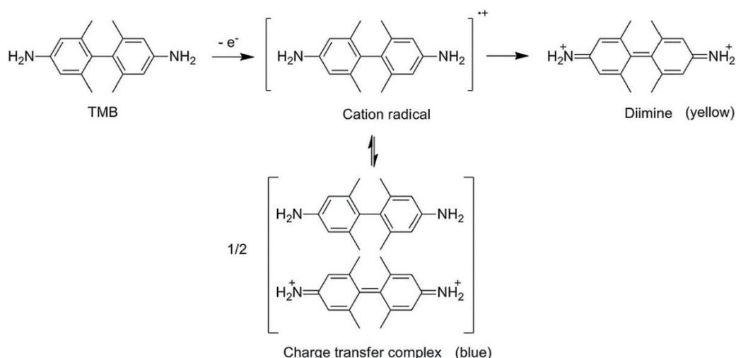
**Figure 3.2:** Schematic representation of two-step TMB conversion reaction (P. D. Josephy et al. 1982).
