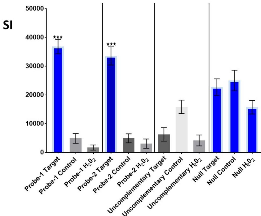
**Figure 3.23:** Signal intensity of LFA in which SiNPs were capped with Probe-1, Probe-2, Uncomplementary Probe and Null (uncapped). LFAs on which complementary targets were applied generated significantly high SI.
