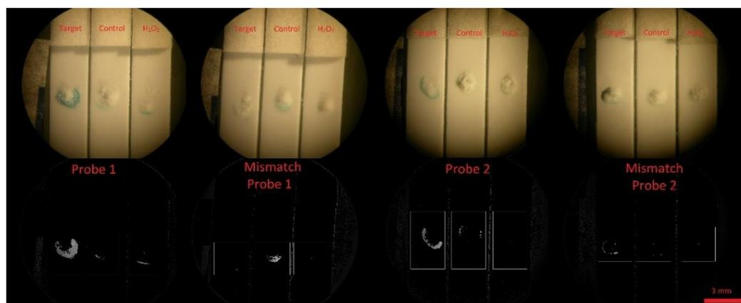
**Figure 3.24:** The image of LFAs including SiNPs capped with Probe-1, Mismatch Probe-1, Probe-2 and Mismatch Probe-2. ([TMB] = 5 mM, 1%  $H_2O_2$ , 0.5 mg/mL of HRP and 37°C)
