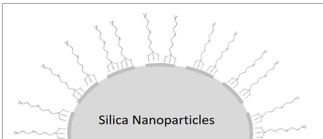
**Figure 3.10:** Representation of required silanization of SiNPs (inspired from Rafael A. Bini, *et al.*, 2011)
