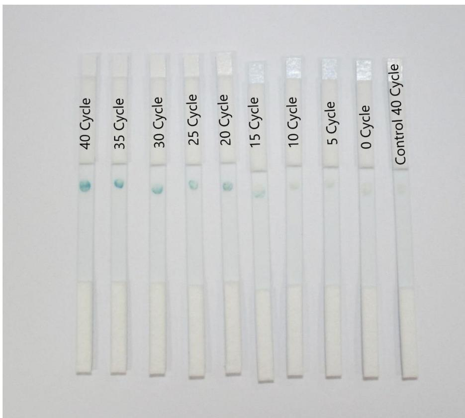
**Figure 3.31:** The overall image of LFAs, including Probe-1 capped SiNPs, onto which, target amplicon with various number of cycle (40, 35, 30, 25, 20, 15, 10, 5, 0) and control amplicon (40 cycle) were applied separately. Until 10 cycle, Signal could be detected on LFAs. ([TMB] = 5 mM, 1% H<sub>2</sub>O<sub>2</sub>, 0.5 mg/mL of HRP and 37°C)
