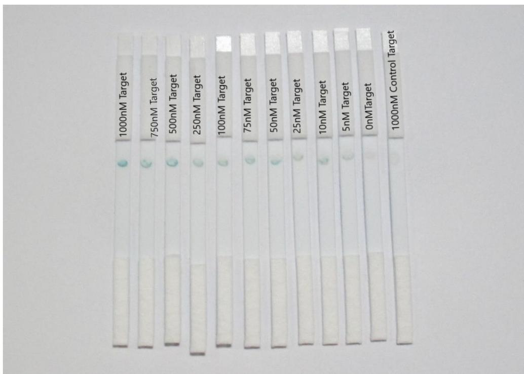
**Figure 3.26:** The overall images of LFAs, including Probe-1 capped SiNPs, onto which, gradual concentration of synthetic complementary Target-1 (1000 nM, 750 nM, 500 nM, 250 nM, 100 nM, 75 nM, 25 nM, 10 nM, 5 nM and 0 nM) and 1000 nM of uncomplementary Control Target were applied. ([TMB] = 5 mM, 1% H<sub>2</sub>O<sub>2</sub>, 0.5 mg/mL of HRP and 37°C)
