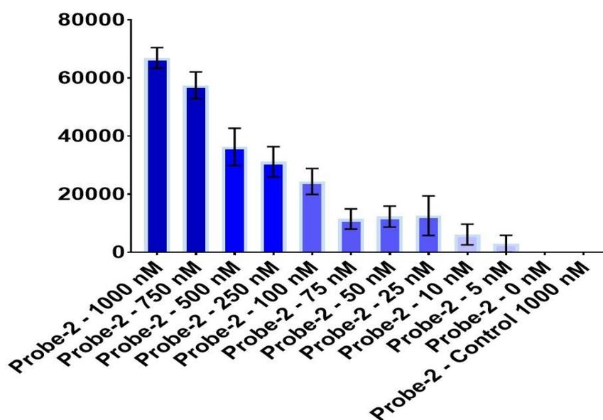
**Figure 3.29:** Signal Intensity of LFAs, including Probe-2 capped SiNPs, onto which, gradual concentration of synthetic complementary Target-2 (1000 nM, 750 nM, 500 nM, 250 nM, 100 nM, 75 nM, 25 nM, 10 nM, 5 nM and 0 nM) and 1000 nM of uncomplementary Control Target.
