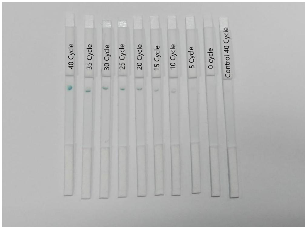
**Figure 3.33:** The overall image of LFAs, including Probe-2 capped SiNPs, onto which, target amplicon with various number of cycle (40, 35, 30, 25, 20, 15, 10, 5, 0) and control amplicon (40 cycle) were applied separately. Until 10 cycle, Signal could be detected on LFAs. ([TMB] = 5 mM, 1%  $H_2O_2$ , 0.5 mg/mL of HRP and 37°C)
