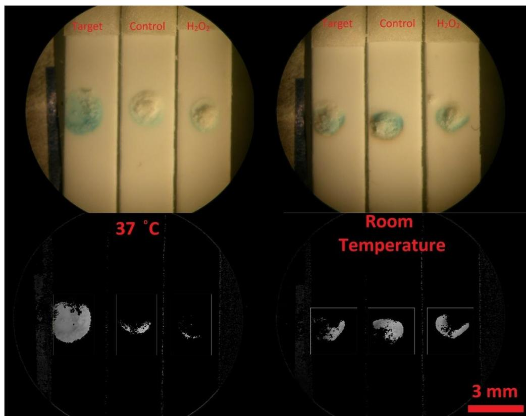
**Figure 3.11:** Photographs of SI on LFA in which SiNPs had been prepared at different temperatures: 37°C and room temperature. ([TMB] = 5 mM, 1% H<sub>2</sub>O<sub>2</sub>, 0.5 mg/mL of HRP)
