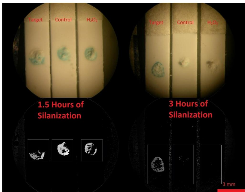
**Figure 3.13:** Images of LFA in which SiNPs were prepared with 1.5 hours and 3 hours silanization. ([TMB] = 5 mM, 1% H<sub>2</sub>O<sub>2</sub>, 0.5 mg/mL of HRP and 37°C)
