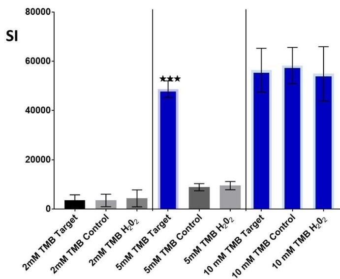
**Figure 3.6:** Signal Intensity (SI) for various TMB concentration (2mM, 5 mM and 10mM) on LFA with Probe-1 capped SiNPs. there was not significant SI on 2mM and 10 mM of TMB (one-way ANOVA,  $P > 0.05$ ,  $n = 3$ ) while LFAs, on which target was applied, significantly differentiated from control and H<sub>2</sub>O<sub>2</sub> (one-way ANOVA, Tukey HSD test,  $P > 0.05$ ,  $n = 3$ ).
