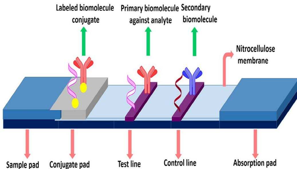
**Figure 1.5:** Representation of Lateral Flow Assay (LFA) components (E. B. Bahadır and M. K. Sezgentürk, 2016)
