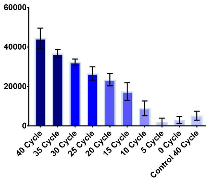
**Figure 3.34:** The graph of SIs on LFAs with Probe-1 capped SiNPs, onto which, target amplicon (20 ng input DNA was added in 50  $\mu$ L PCR solution) with various number of cycle (40, 35, 30, 25, 20, 15, 10, 5, 0) and control amplicon (40 cycle) were applied separately. Until 10 cycle, LFAs could response complementary targets. LoD was determined as 15 Cycle.
