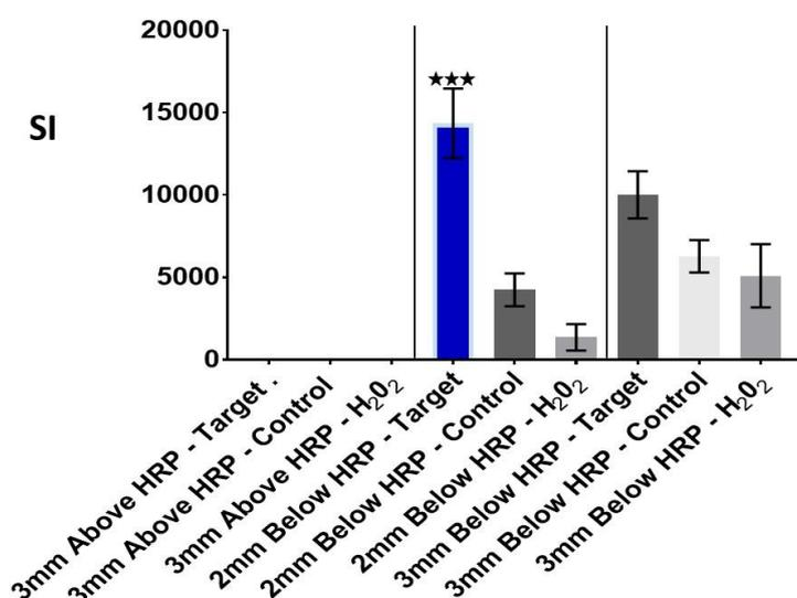
**Figure 3.20:** Signal intensity of LFA in which HRPs were posited on different locations: 3 mm above SiNPs, 2 mm below SiNPs and 3 mm below SiNPs. HRP 3 mm above SiNPs could not generate signal. HRP 2 mm below SiNPs significantly recognize target (one-way ANOVA, Tukey HSD test,  $P < 0.001$ ,  $n = 3$ ).
