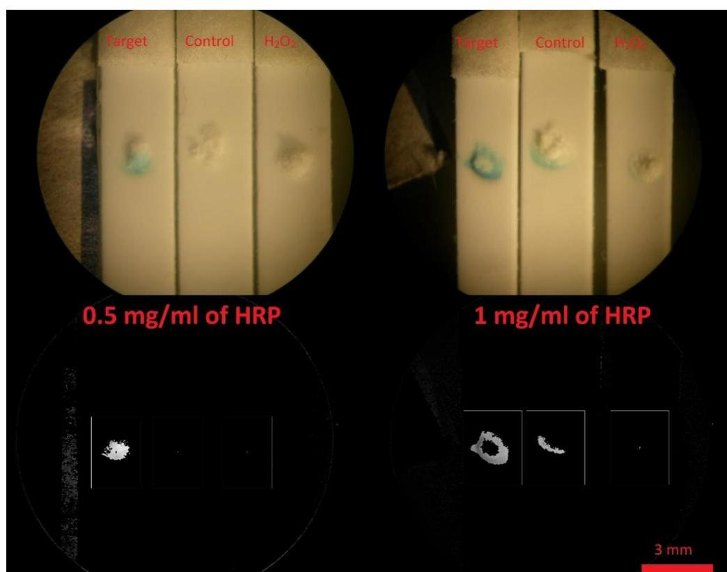
**Figure 3.7:** The response of LFAs for 0.5 mg/mL and 1 mg/mL of HRP ([TMB] = 5 mM, 1% H<sub>2</sub>O<sub>2</sub>, and room temperature)
