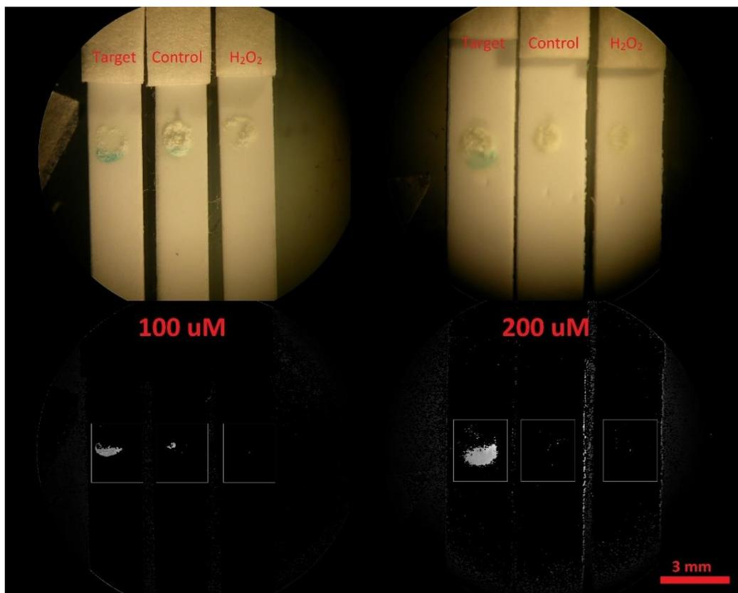
**Figure 3.15:** The images of LFA in which SiNPs were capped with 100uM and 200uM of oligonucleotide probes. ([TMB] = 5 mM, 1% H<sub>2</sub>O<sub>2</sub>, 0.5 mg/mL of HRP and 37°C)
