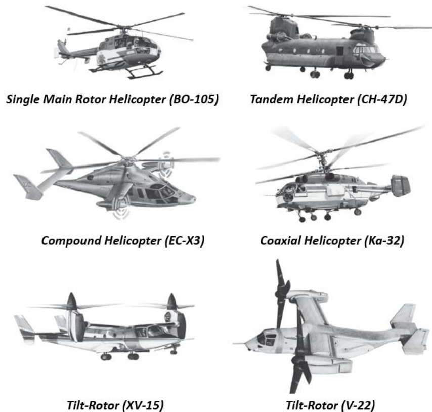
Figure 2-8 Different Types of Rotorcraft Configurations [30]
