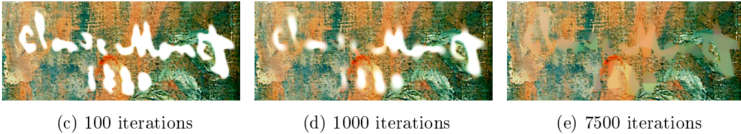
Figure 3.17: (a) Original Image. (b) Region mask \Lambda . (c-e) Inpainted Image for different numbers of inpainting iterations on 145x349 pixels using Bertalmio Image Inpainting [21]
