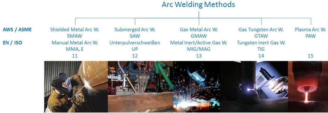
Figure 13. Classification of arc welding methods according to the standards [1].
