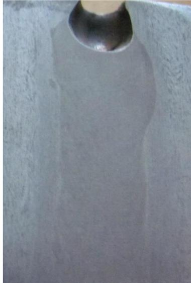
*Figure 23. Real illustration of key-hole based HPA welded steel.*
